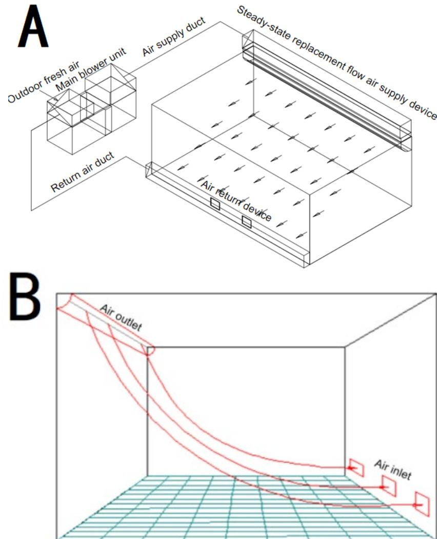
**Fig. 1.** (A) Schematic of the steady-state replacement flow air supply system. (B) Schematic of its working principle.
