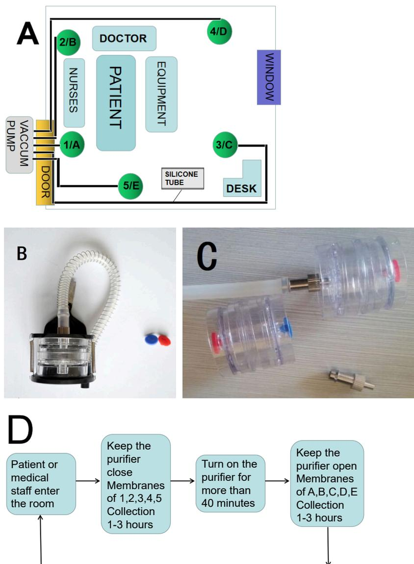
**Fig. 2.** (A) Placement of the sampling membranes in the bronchoscopy room; (B, C) Equipment for installing the membrane: the sampling clamp; (D) Sampling flowchart.
