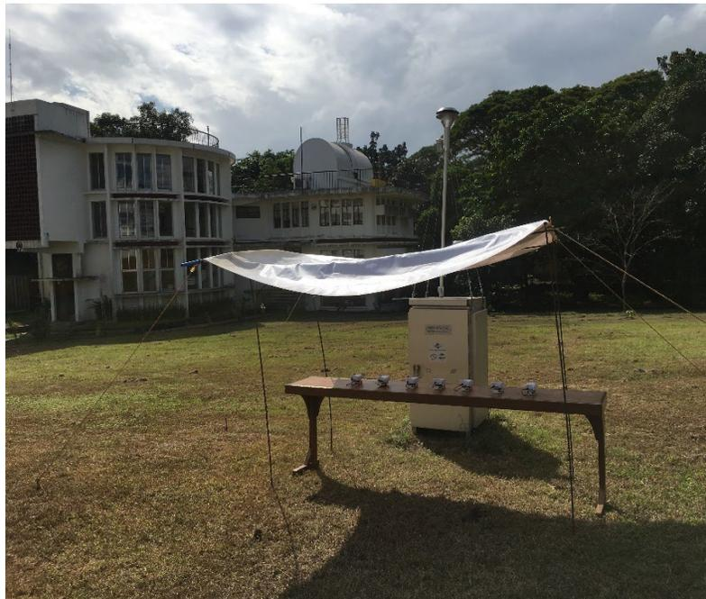
**Figure S2.** Collocation experiment of the AS-LUNG sensors (on table) at the Manila Observatory, with the beta-attenuation monitor (BAM) behind.
