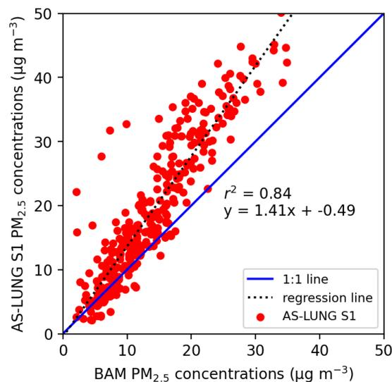
**Figure S3.** Scatter plot shows the observed relationship between an AS-LUNG sensor (Sensor 1) measurements against those from the Beta Attenuation Monitor (BAM) during the 16-day collocation experiments at the Manila Observatory site from 27 March to 12 April 2019.
