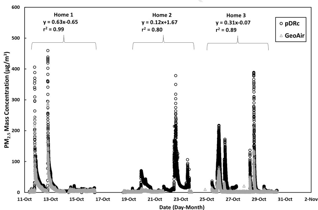
Figure 6. Time series plot of the filter-corrected pDR-1500 measurements and GeoAir2 measurements in three different indoor residential environments.
