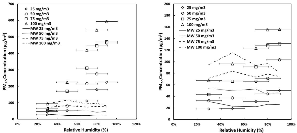
Figure 5: Relative humidity (%) effects on  $PM_{2.5}$  concentrations ( $\mu g m^{-3}$ ) detected by the a) OPC-N3 and b) GeoAir2 compared to the MiniWRAS (MW)  $PM_{2.5}$  concentration at different steady states of salt aerosol. The MW was not affected by the humidity because the particles were dried before measurements were performed.
