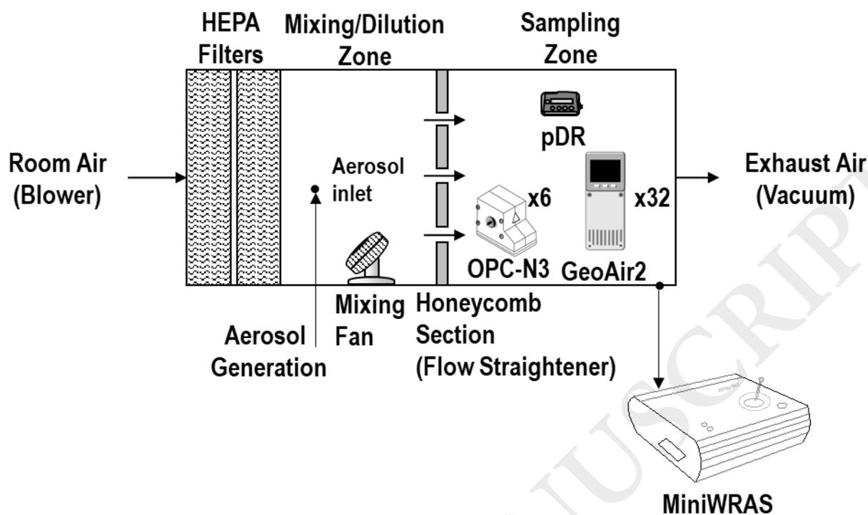
Figure 1. The experimental chamber used to test the sensors for salt and dust particulate matter detection.
