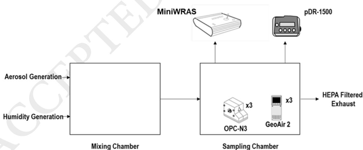
Figure 2. Experimental chamber designed to test the effects of different relative humidity levels on sensor reading of particulate mass.
