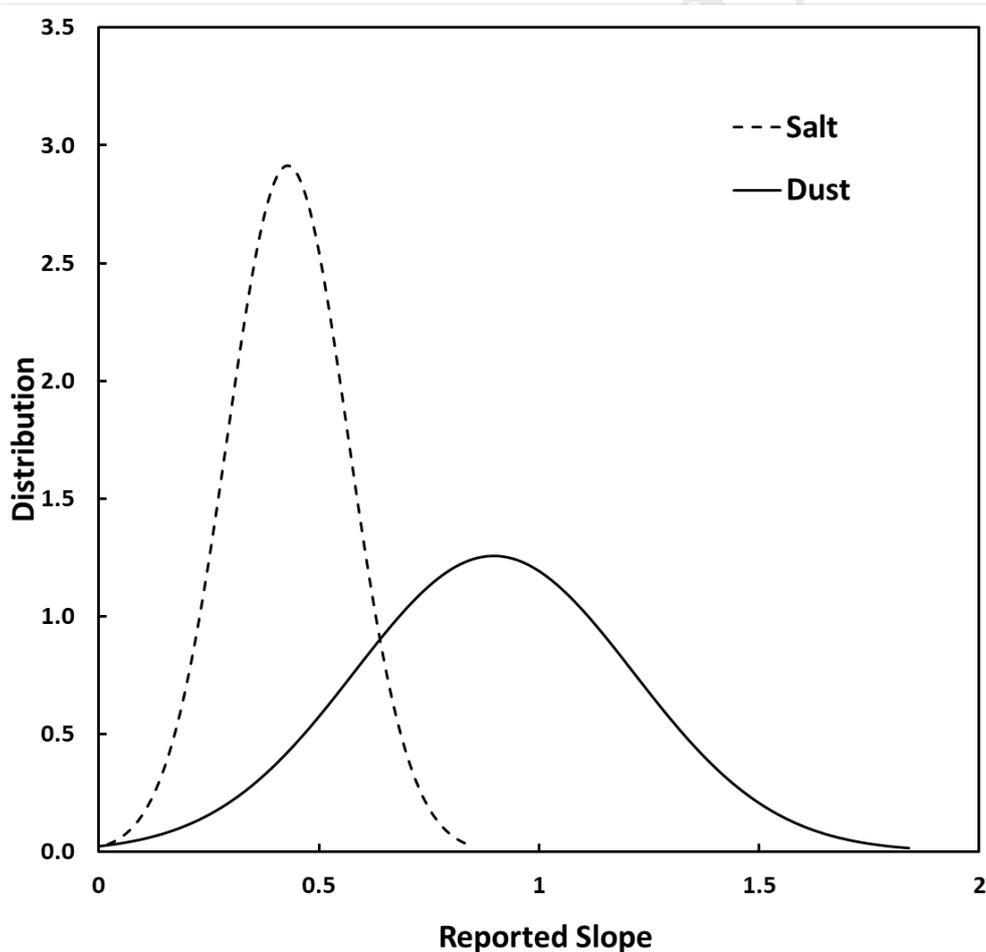
Figure 4. The normal distribution of slopes was recorded by the GeoAir2 units across all salt aerosol testing.
