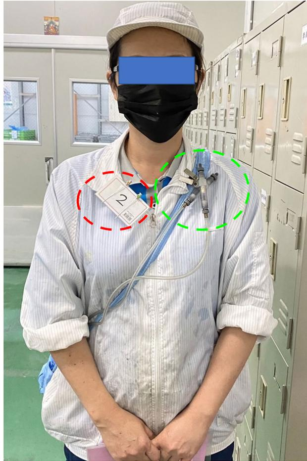
**Fig. 2.** Worker wore two types of samplers for monitoring the VOC exposure. Left red circle: needle trap samplers; right green circle: charcoal adsorption tubes.
