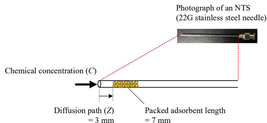
**Fig. 1.** Schematic configuration of needle trap samplers.
