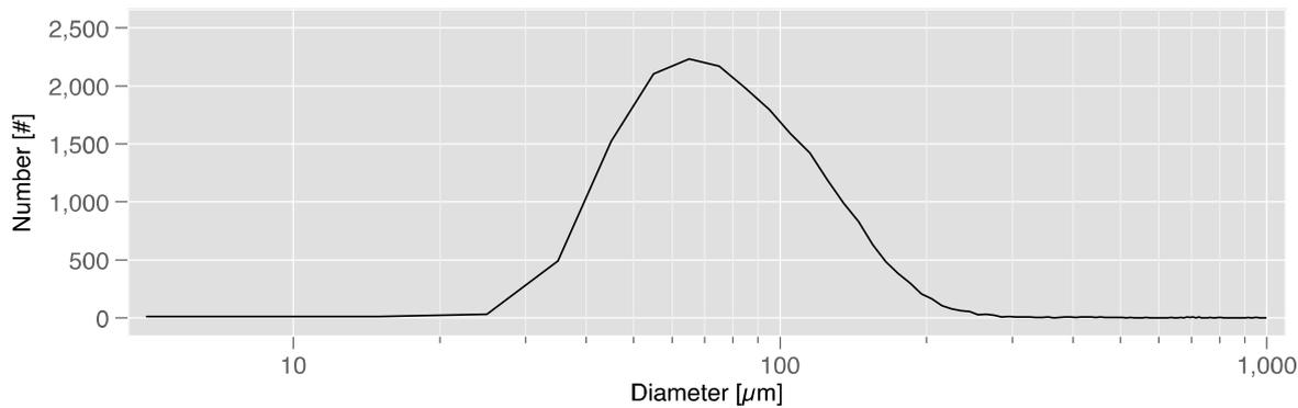
**Fig. 2.** Size distribution of the spray generated by the 1.3 mm mist nozzle at 3 bar pressure.
