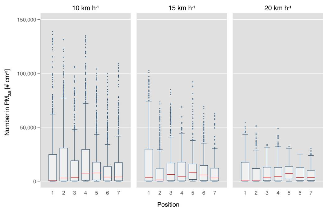
**Fig. 3.** Box plot of the number concentrations in the  $\text{PM}_{2.5}$  size range measured at different positions and speed. Positions: 1 and 2: left and right in front row; 3, 4 and 5: left, middle and center of second row; 6 and 7: left and right of back row.
