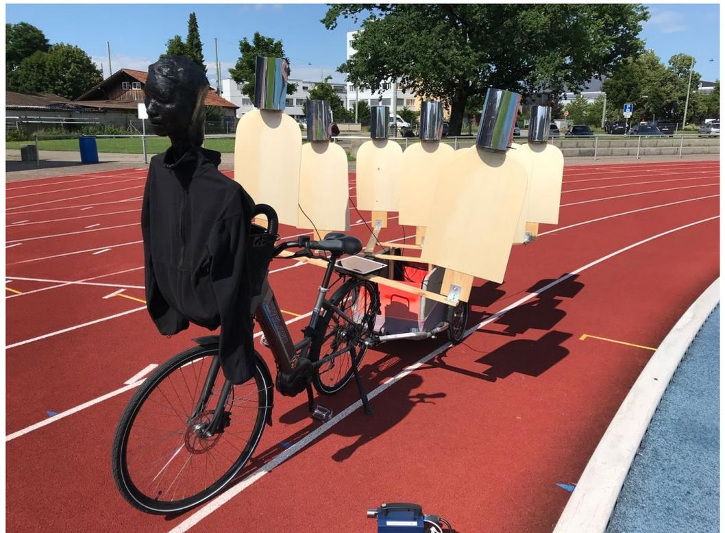
**Fig. 1.** Arrangement of the dummies, here shown with the fog-emitting source.
