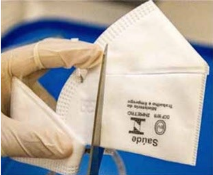
Figure S2. Detail of the respirator cutout in the contact region of the user's nose and mouth to study the microbiota.
