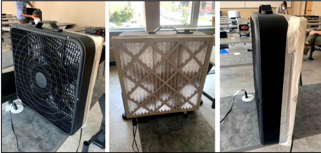
Figure S3 Low-cost portable mitigation device: a standard box fan with a MERV13 filter taped to the intake side of the fan.
