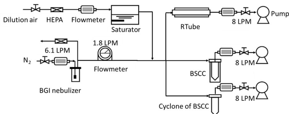
**Fig. 3.** Experimental setup for testing Phi6 infectivity conservation efficiency.
