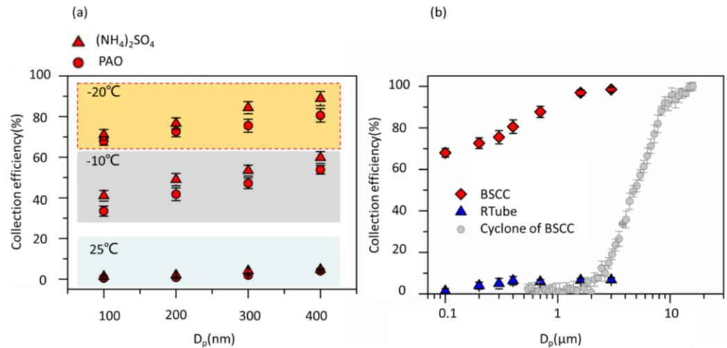
**Fig. 4.** Collection efficiencies as a function of aerodynamic diameter for: (a) BSCC at condensation temperatures of  $-20$ ,  $-10$  and  $25^\circ\text{C}$ . (b) Cyclone (using NaCl aerosols), BSCC and RTube (using PAO aerosols with diameters of 100, 200, 300 and 400 nm and PSL spheres with diameters of 0.7, 1.6 and 3  $\mu\text{m}$ ) at the condensation temperature of  $-20^\circ\text{C}$ . Error bars represent the standard deviations of three measurements.
