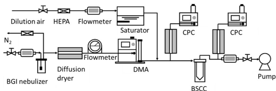
**Fig. 2.** Experimental setup for collection efficiency tests.
