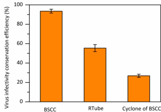
**Fig. 5.** Phi6 infectivity conservation efficiency of the BSCC, RTube and cyclone of BSCC. Error bars represent the standard deviations of three measurements.
