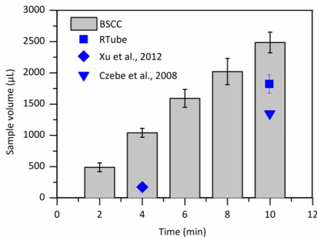
**Fig. 6.** Volumes of samples collected by the BSCC, RTube and some exhaled breath samplers in previous studies. Error bars represent the standard deviations of three measurements.
