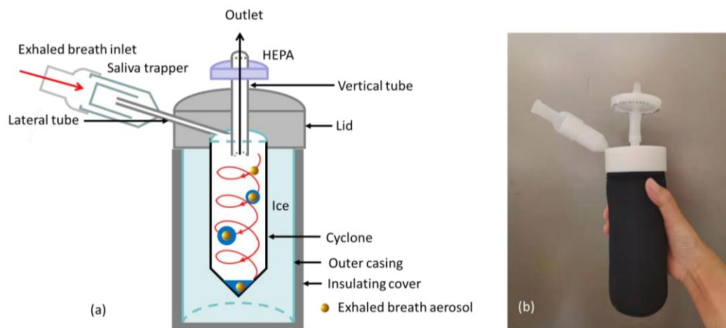
**Fig. 1.** (a) Schematic and (b) photograph of the BSCC.
