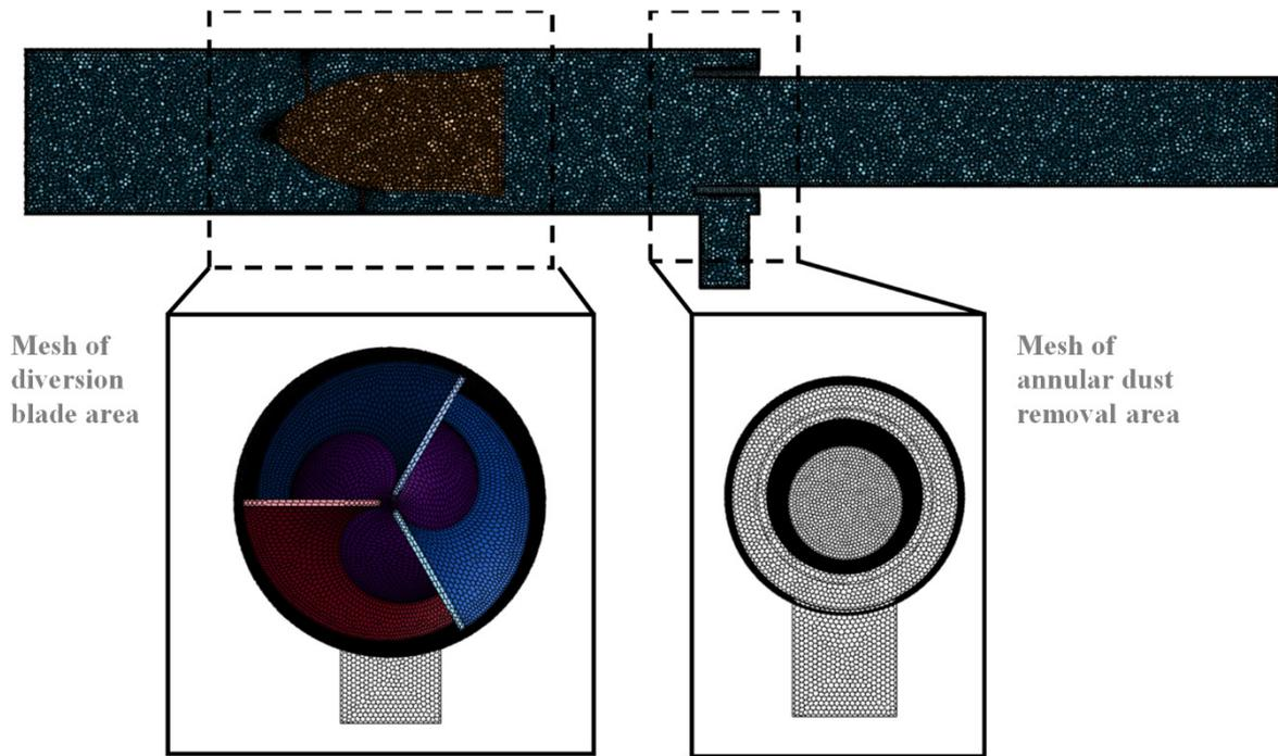
**Fig. S1.** A polyhedral shape mesh for numerical simulation.
