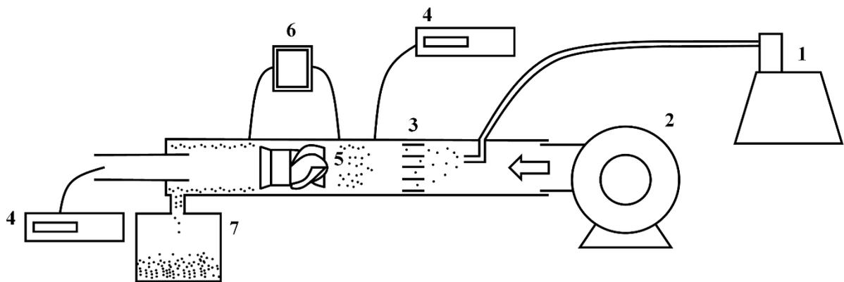
**Fig. S2.** Schematic of the system. (1) dust generator, (2) main blower, (3) honeycomb, (4) dust monitors, (5) cyclone, (6) differential pressure gauge, and (7) dust box.
