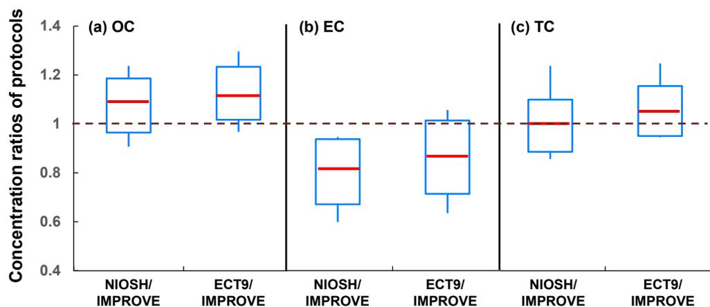
**Fig. 1.** Comparison of the relative (a) OC, (b) EC and (c) TC concentrations measured by the NIOSH and ECT9 protocol with respect to IMPROVE. The edges of boxes indicate the 25<sup>th</sup> and 75<sup>th</sup> percentile, the whiskers extend to the 10<sup>th</sup> and 90<sup>th</sup> percentile, and the central (red) lines on the boxplots are averaged data.
