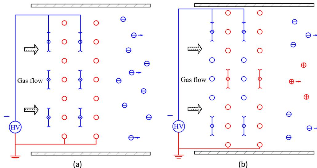
**Fig. 2.** Geometries of the (a) unipolar precharger and (b) bipolar precharger.
