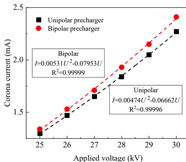
Fig. 8.  $V-I$  characteristics of the unipolar and bipolar prechargers.
