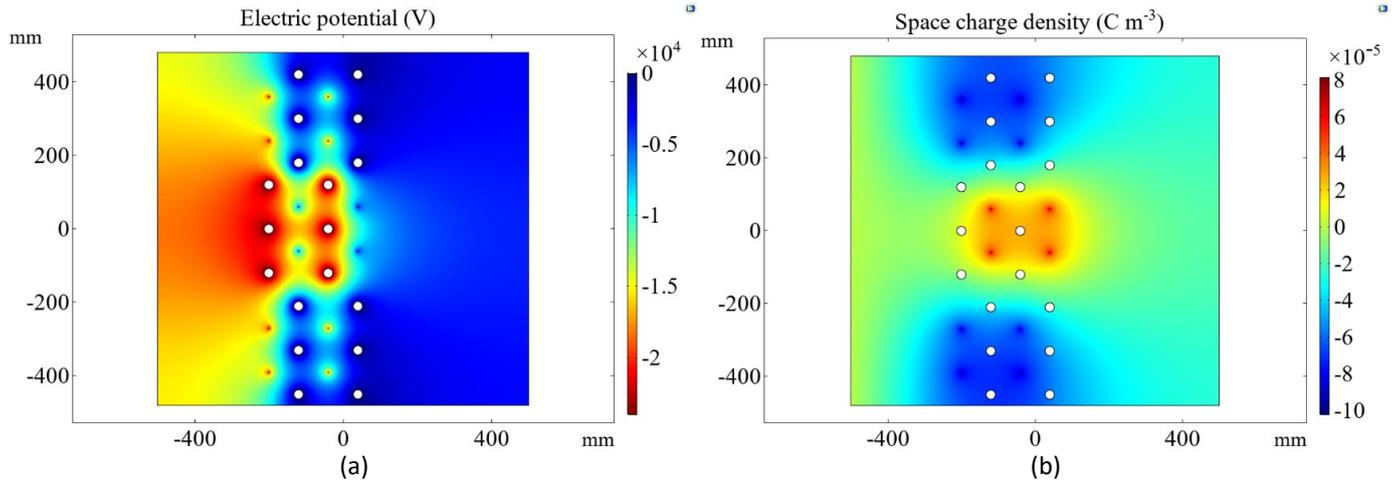
Fig. 4. Electric field distributions in the bipolar precharger: (a) electric potential and (b) space charge density.
