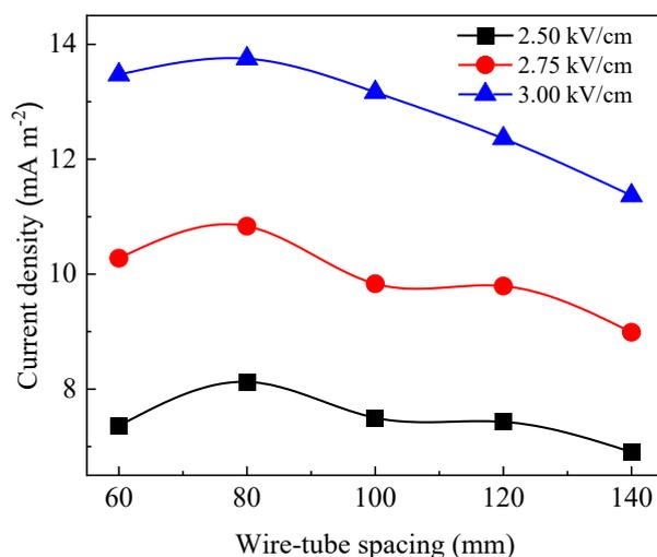
Fig. 6. Relationship between the current density and the wire-tube spacing ( $D = 25$  mm).
