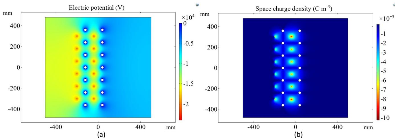
**Fig. 3.** Electric field distributions in the unipolar precharger: (a) electric potential and (b) space charge density.
