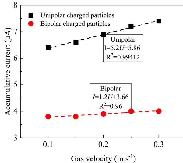
**Fig. 10.** Current produced by charged particles in different gas velocity.
