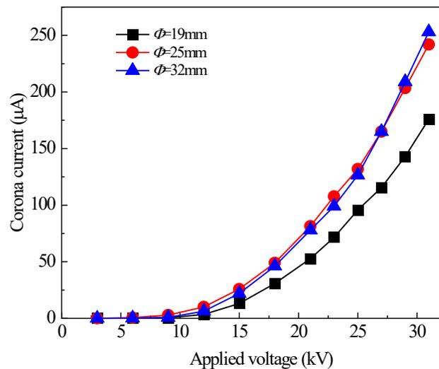
Fig. 7.  $V-I$  characteristics of the BWTE ( $b = 80$  mm).
