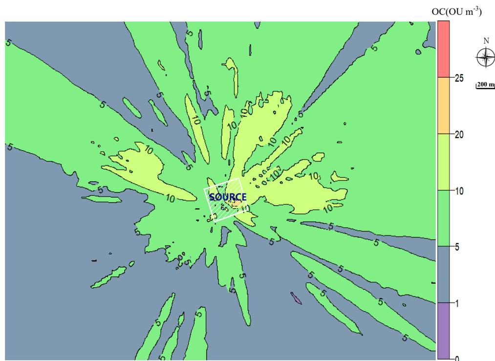
**Fig. 2.** The result of the odor dispersion simulation using the Aermol model system.
