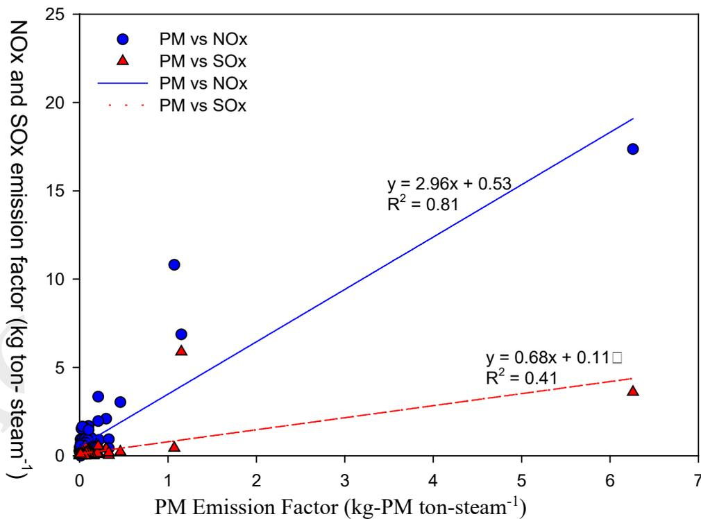
**Figure 4b** Relationships of PM emission factor with NOx and SOx based on steam generation
