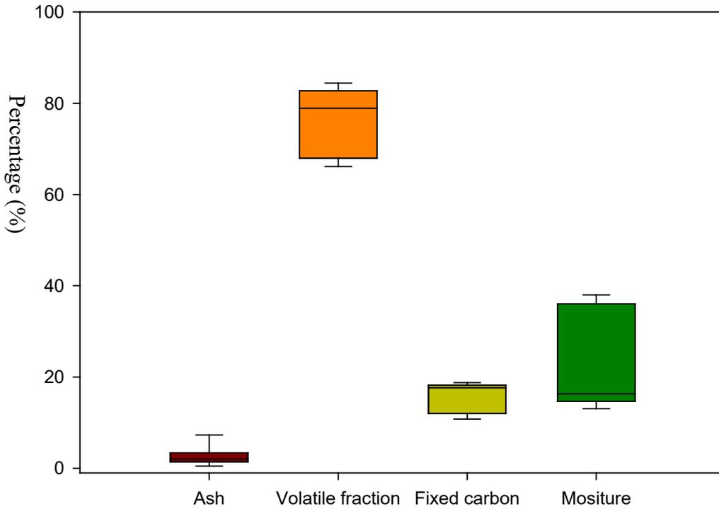
**Figure 2a** Approximately analysis of waste woods from 100 industrial-sized wood combustion boilers
