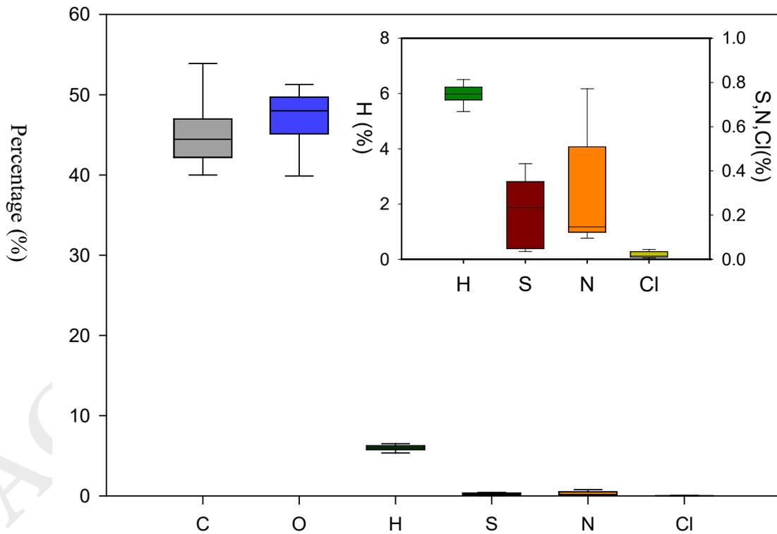
**Figure 2b** Elemental constituents of waste woods from 100 industrial-sized wood combustion boilers
