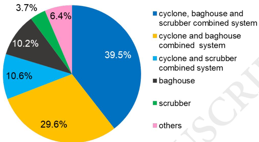
**Figure 5** Air pollution control system of waste combustion boiler
