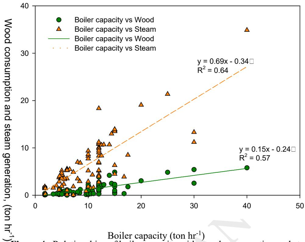
**Figure 4a** Relationships of boiler capacity with wood consumption and steam generation
