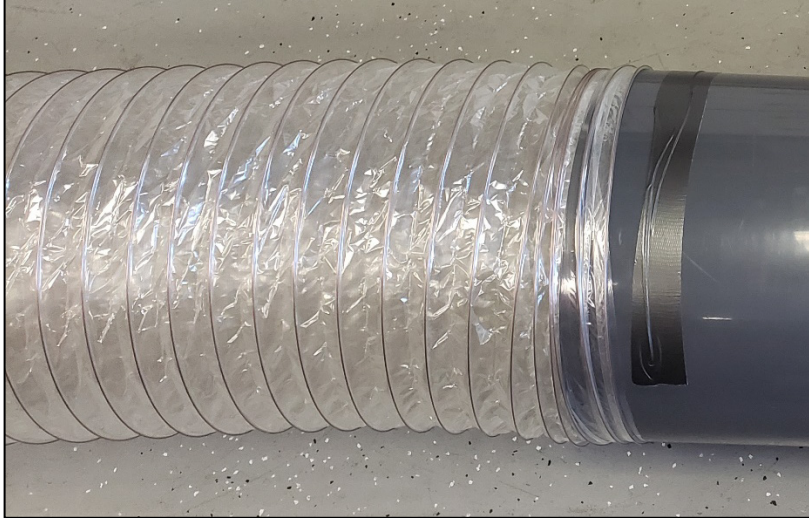
Fig. S2. Photograph of the Mylar tubing used to construct the fog-and-tube scrubber apparatus.
