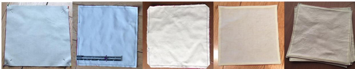
Fig. S2. Wash/dry sample coupon fabrication steps. (a) 8" squares are cut from the two different fabrics, and one of each color are placed right sides together (b) a 1/4" seam is stitched around the edges, leaving a ~2" gap for flipping inside out (c) corners are clipped to remove bulk (d) sample coupon is flipped inside out and pressed into shape (e) topstitching around the outside edge to enclose raw edges and reinforce seams.
