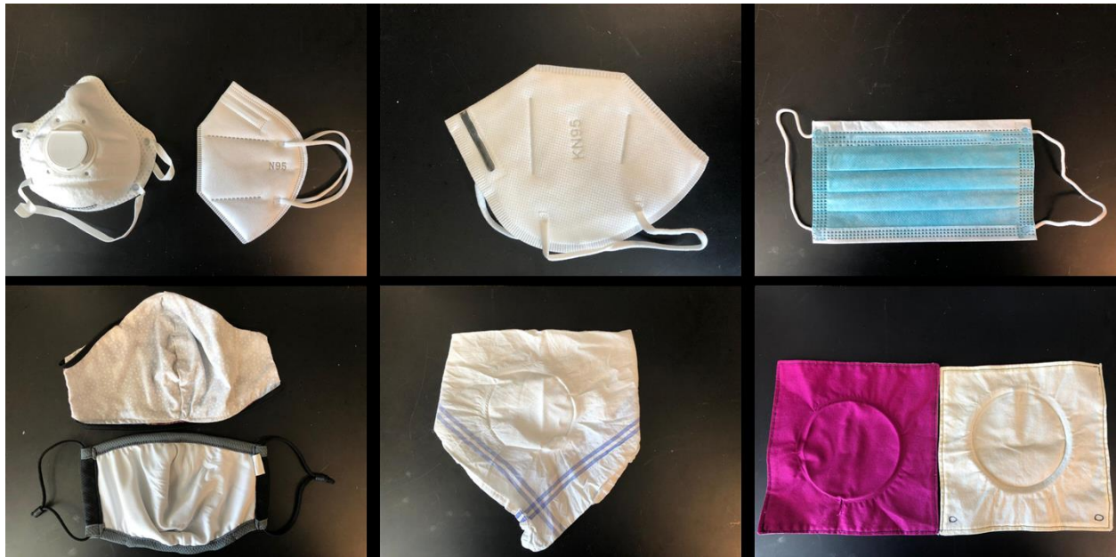
Fig. S1. Different samples that were used in this study are shown from top right to bottom in clockwise direction: N95 respirator, KN95 respirator, Surgical mask (SM), wash/dry sample coupon, 2-ply bandana and Cloth mask (CM).
