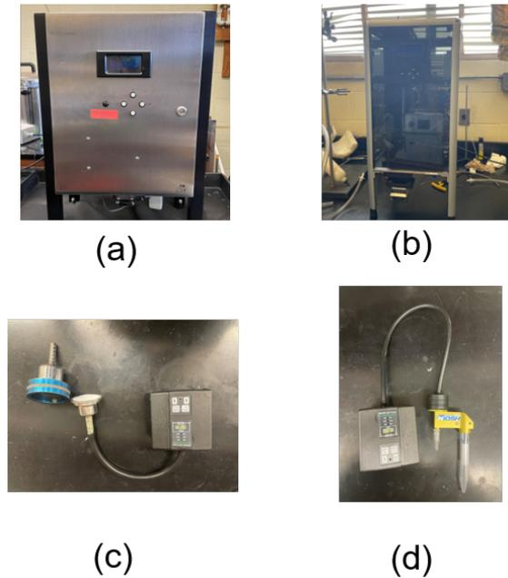
Figure S1. Four samplers deployed to collect air samples in the fitness center: (a) BioSpot-VIVAS; (b) VIVAS; (c) an in-line holder for PTFE filter; (d) NIOSH BC-251 bioaerosol sampler.
