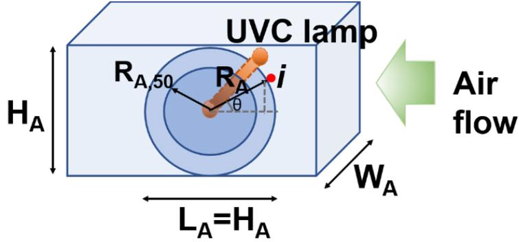
Figure S3. Schematic figure of UVC dose in the UVGI inside AHU
