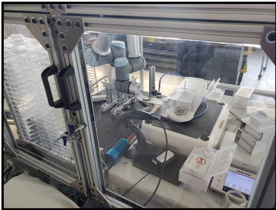
Figure S1: Example photos of the AIRLIFT weighing system. (Top) Image of AIRLIFT system in the Advanced Aerosol Laboratory at Colorado State University. (Bottom) Image showing the robotic arm about to neutralize a filter using the radiation source and then deposit the filter on the microbalance. The filter storage rack can be seen in the left edge of the photo.
