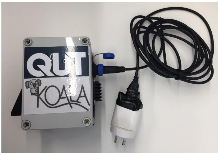
Fig S1(b) KOALA modified for use via the mains and USB cable.
