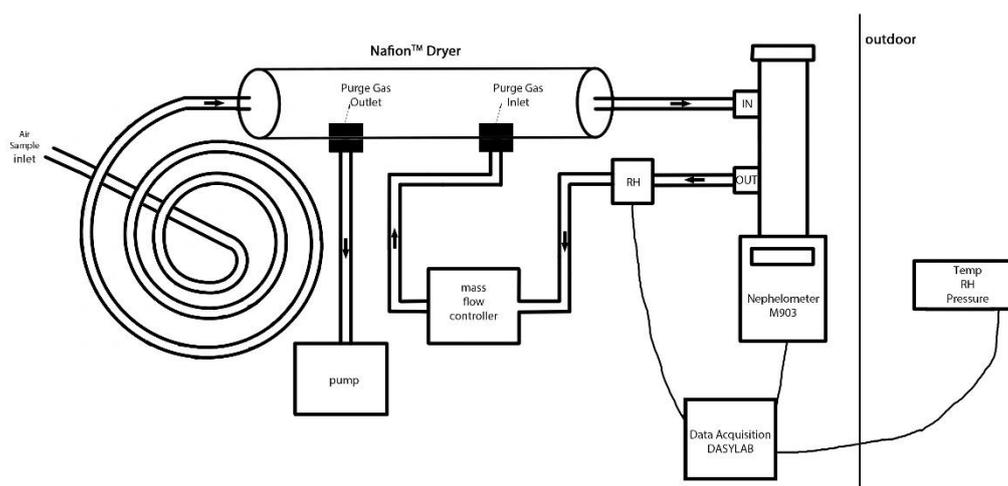
**Fig. S1.** RRN-903 set up with the Nafion™ drier in place.
