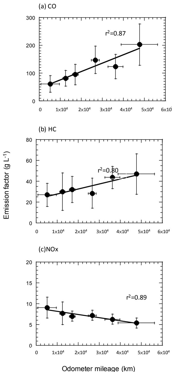
**Fig. 3.** Emission factors of (a) CO, (b) HC, and (c) NO<sub>x</sub> of selected motorcycles with various running mileages.
