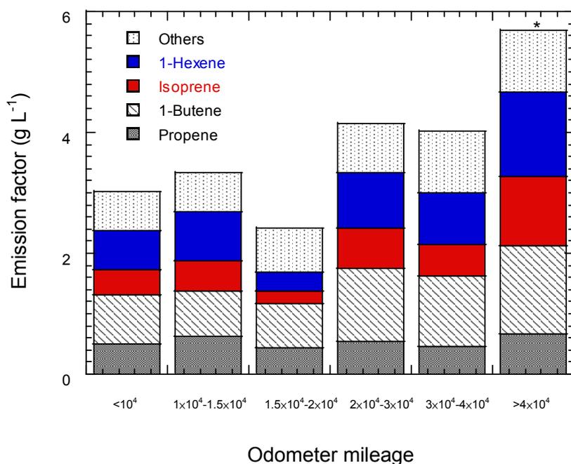
**Fig. 5(b).** Emission factors of dominant olefins of selected motorcycles for different running mileage (significance versus group with mileage < 10,000 km: \* $p < 0.05$ ).
