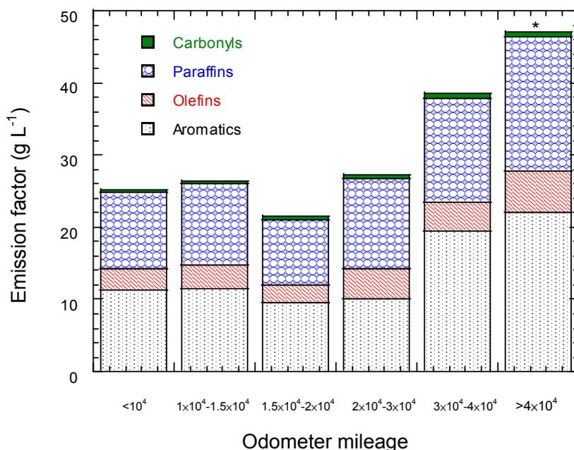
**Fig. 4.** Emission factors of paraffins, olefins, aromatics, and carbonyls for selected motorcycles with various running mileages (significance versus group with mileage < 10,000 km: \* $p < 0.05$ ).
