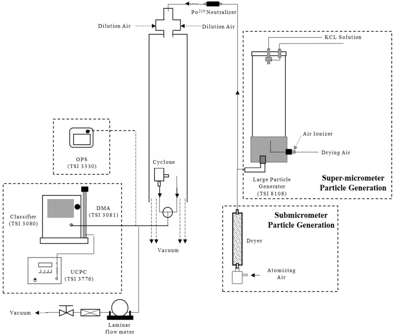
Fig. 2. Schematic diagram of experimental setups for measuring the particle penetration of prototype cyclones.
