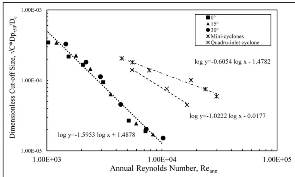
**Fig. 8.** The correlation of dimensionless particle cut-off size to annular flow Reynolds number for studied cyclones. The correlations for mini-cyclone and quadru-inlet cyclone are also included.
