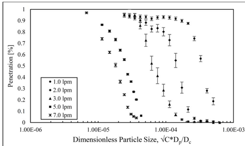
**Fig. 6(a).** The particle penetration as a function of dimensionless particle size for the cyclone with 30° contraction angle at different operational flow rates.
