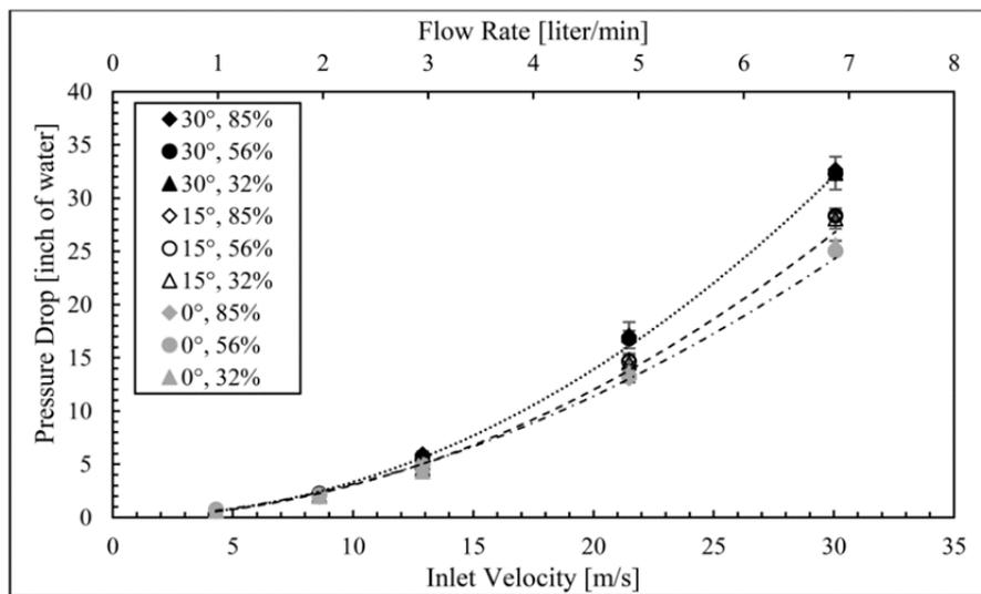
Fig. 3. Measured pressure drop as a function of cyclone inlet velocity of studied cyclones.
