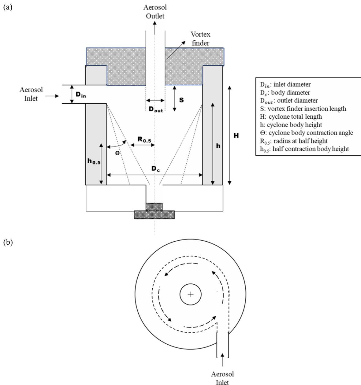
**Fig. 1.** Schematic diagram of studied cyclones with conical contraction body: (a) side cross-sectional view; (b) top cross-sectional view.
