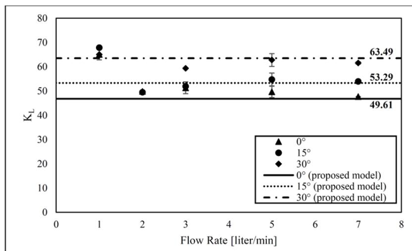
**Fig. 4.** The comparison of the measured and calculated loss coefficients ( $K_L$ ) as a function of cyclone inlet velocity for the prototype cyclones (calculated by the revised Dirigo model).
