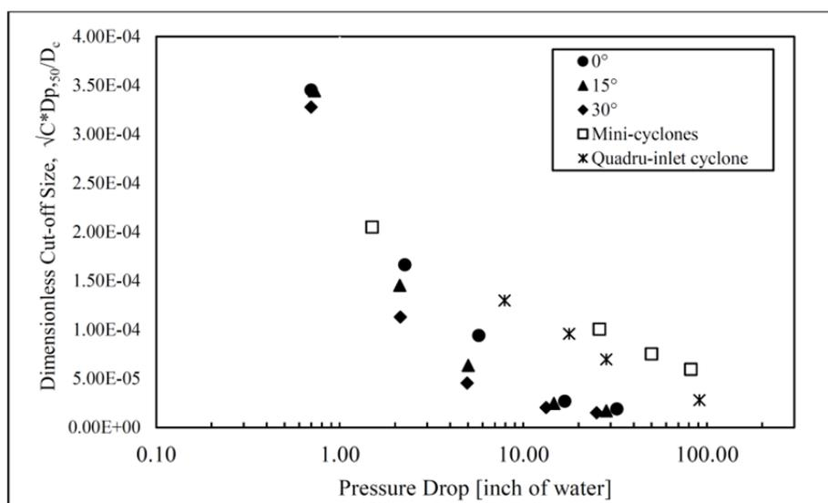
**Fig. 9.** The correlation between dimensionless cut-off size and cyclone pressure drop for studied cyclones, mini-cyclone and quadru-inlet cyclone.
