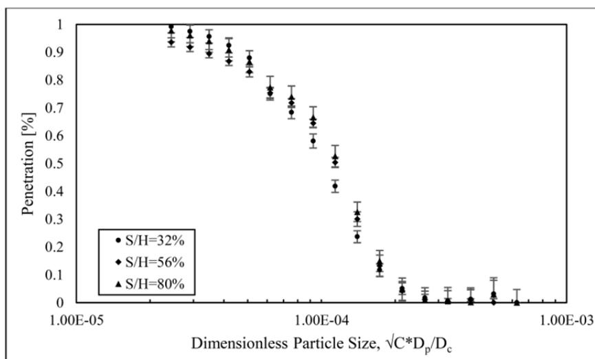
**Fig. 7.** The particle penetration as a function of dimensionless particle size for prototype cyclones having different insertion length of vortex finder tube.
