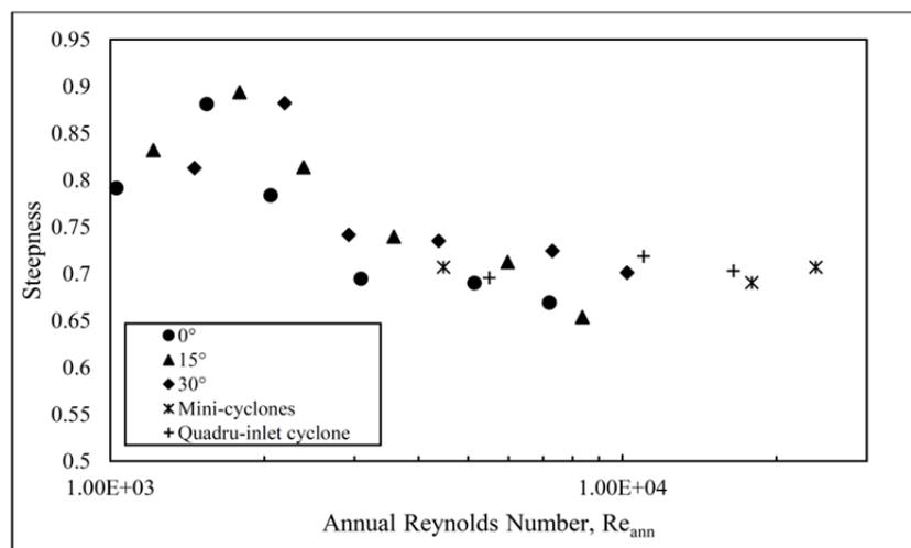
**Fig. 6(b).** The steepness of cyclone penetration curves as a function of cyclone flow rate for studied cyclones, mini-cyclones and quadru-inlet cyclone.
