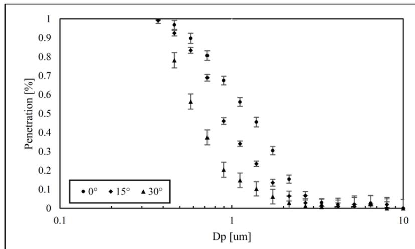
**Fig. 5.** The particle penetration as a function of aerodynamic particle size for prototype cyclones with different body contract angles (operated at 3.0 L min<sup>-1</sup> flow rate).
