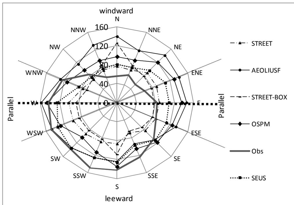
**Fig. 4.** Pollution rose of observed NO<sub>x</sub> concentrations (ppb) at Cordoba Avenue sampling site, and calculated with STREET, OSPM, AEOLIUSF, STREET BOX and SEUS models. The dotted black line represents the urban street canyon orientation.
