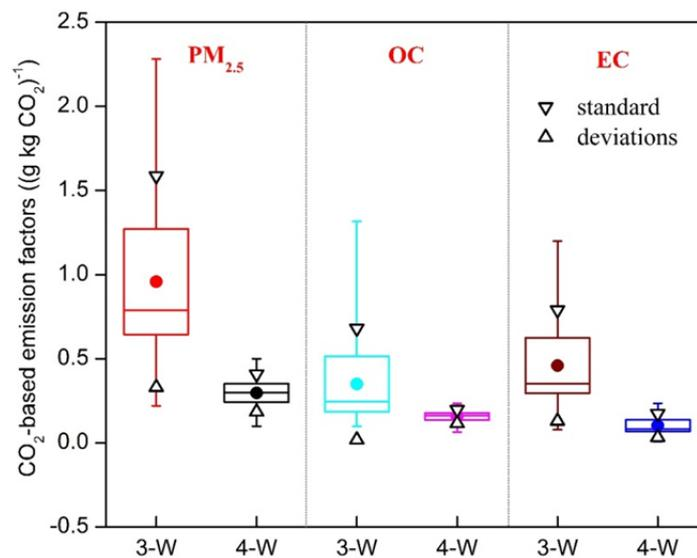
**Fig. 5.** CO<sub>2</sub>-based EFs of PM<sub>2.5</sub>, OC, and EC for RVs. The box shows the interquartile range, line in the box shows the median, and circle shows the mean. The box range represent the upper 25% and lower 25%, and the whiskers represent the maximum and minimum EFs of PM<sub>2.5</sub>, OC, and EC.
