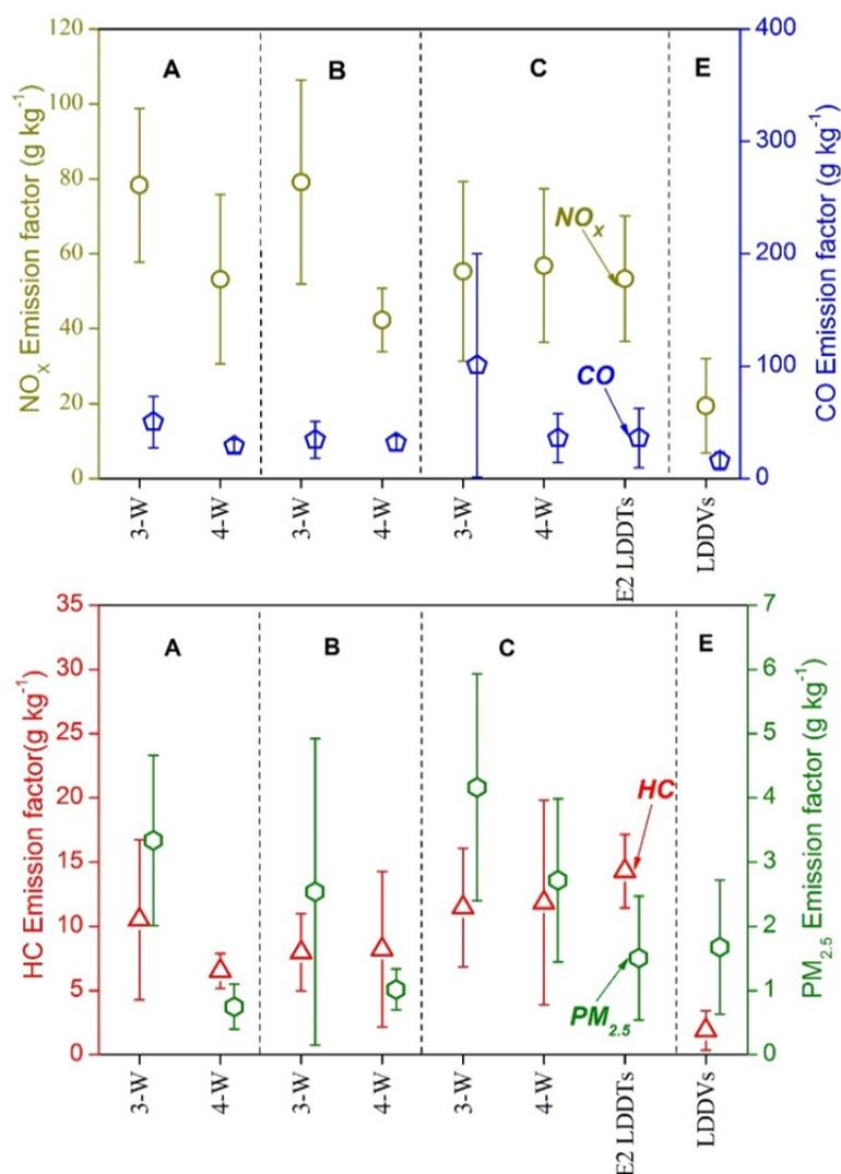
**Fig. 3.** Fuel-based emission factors ( $\text{g kg}^{-1}$ ) of RVs, LDDTs, and LDDVs (error bars show standard deviations). A: The Pre-China II RVs in this study; B: The China II RVs in this study C: Yao *et al.* (2011a) (Pre-China II RVs); E: Chiang *et al.* (2012); E2: Euro II;
