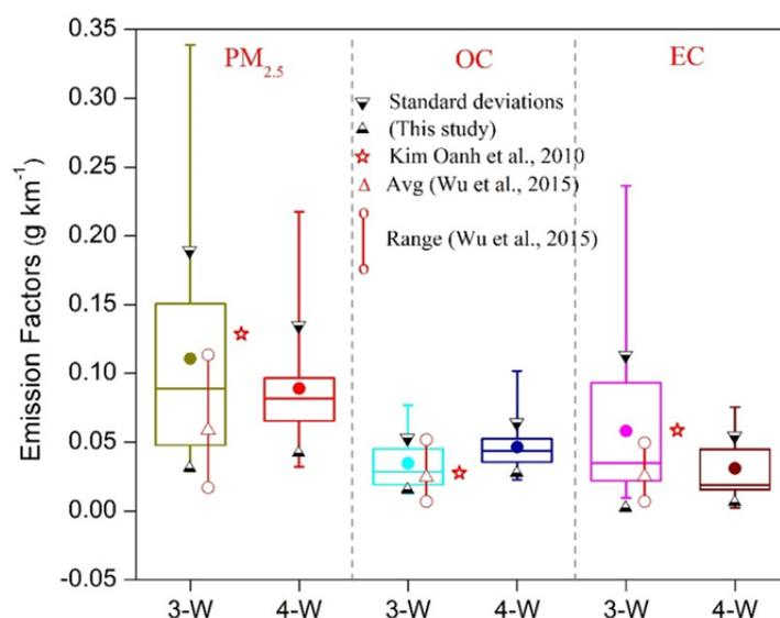
**Fig. 4.** Distance-based EFs of  $PM_{2.5}$ , OC, and EC in various studies. The box shows the interquartile range, line in the box shows the median, and circle shows the mean. The box range represent the upper 25% and lower 25%, and the whiskers represent the maximum and minimum EFs of  $PM_{2.5}$ , OC, and EC.
