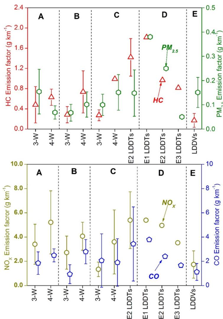
**Fig. 2.** Distance-based emission factors ( $\text{g km}^{-1}$ ) of RVs, LDDTs, LDDVs (error bars show standard deviations). A: The Pre-China II RVs in this study; B: The China II RVs in this study; C: Yao *et al.* (2011a) (Pre-China II RVs); D: Shen *et al.* (2015); E: Chiang *et al.* (2012); E1: Euro I; E2: Euro II; E3: Euro III.
