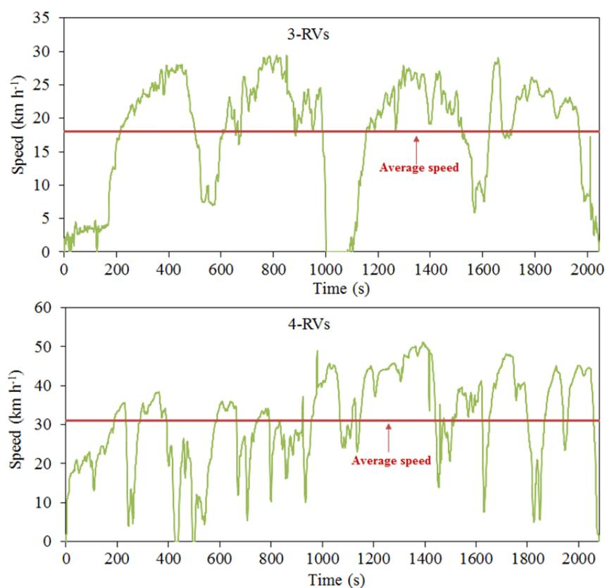
**Fig. 1.** Typical example of velocity profiles of 3-W RVs and 4-W RVs.
