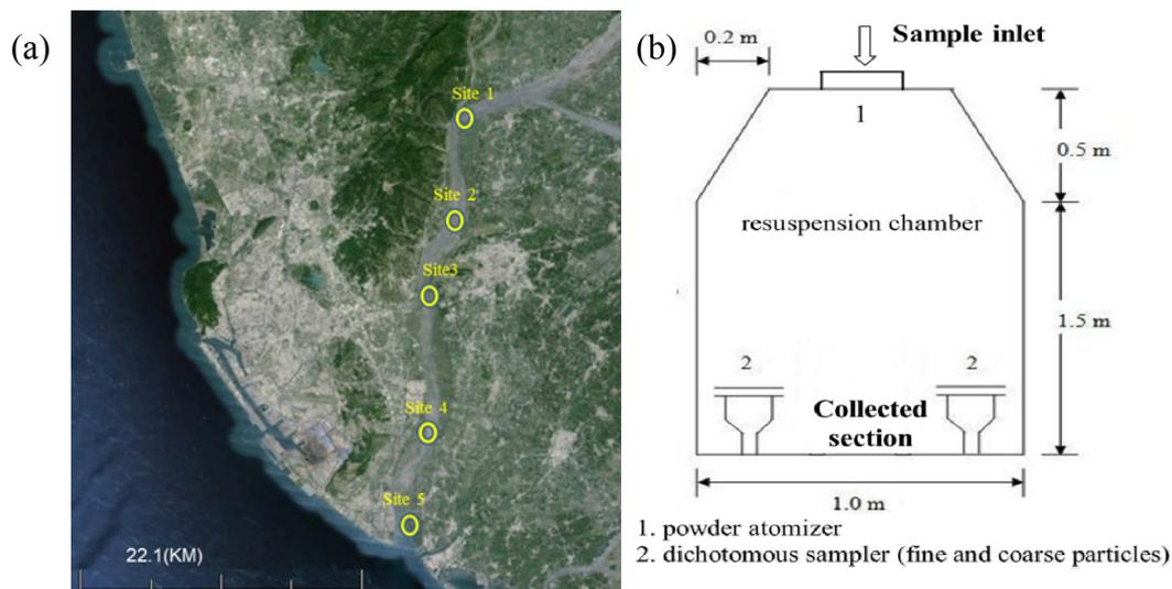
Figure S2 (a) Location of sites for collecting topsoil samples along Kaoping River. (b) Resuspension chamber used for collecting re-suspended fine ( $PM_{2.5}$ ) and coarse ( $PM_{2.5-10}$ ) particles.
