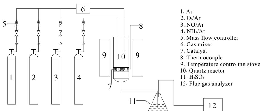
**Fig. 1.** Schematic diagram of the SCR of NO by NH<sub>3</sub> over different nanoporous  $\alpha$ -Fe<sub>2</sub>O<sub>3</sub> catalysts.
