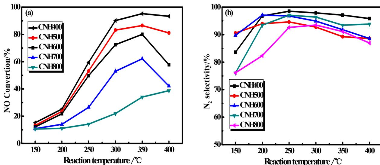
Fig. 2. SCR performances of different nanoporous  $\alpha\text{-Fe}_2\text{O}_3$  catalysts: (a) NO conversion and (b)  $\text{N}_2$  selectivity. (Reaction conditions: NO 500 ppm,  $\text{NH}_3$  500 ppm,  $\text{O}_2$  3 vol%, and balance of Ar, GHSV = 72,000  $\text{h}^{-1}$ ).
