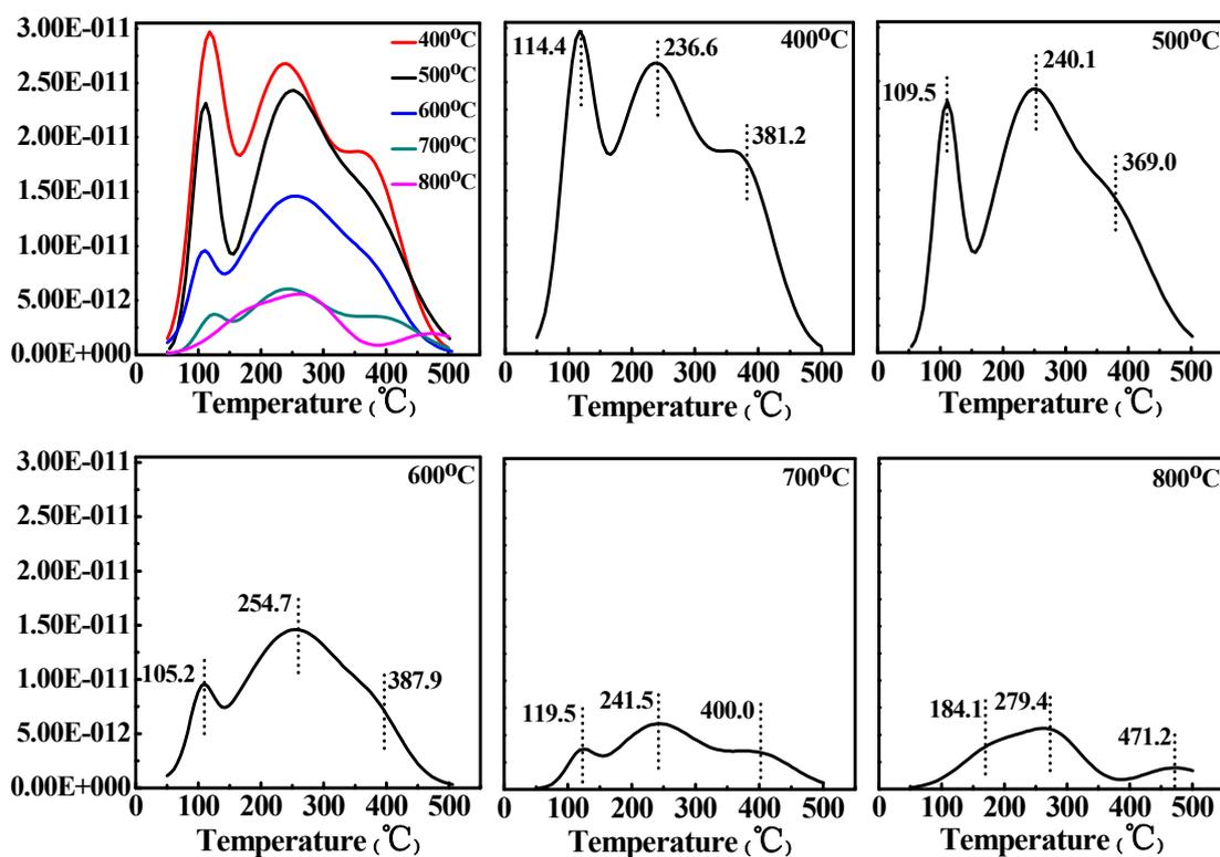
Fig. 8.  $\text{NH}_3$ -TPD curves of various nanoporous  $\alpha\text{-Fe}_2\text{O}_3$ .
