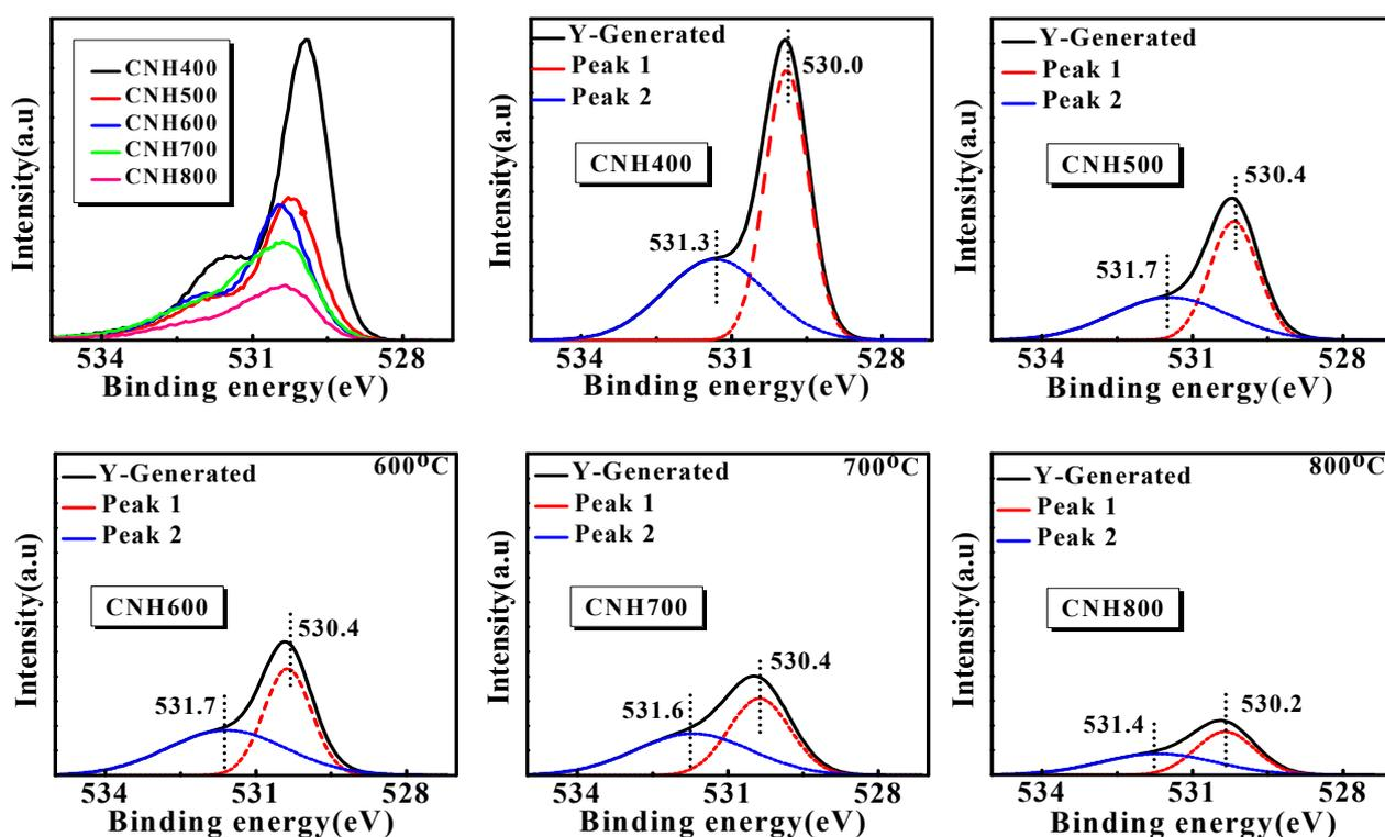
**Fig. 7.** XPS results of O 1s of various nanoporous  $\alpha$ -Fe<sub>2</sub>O<sub>3</sub>.
