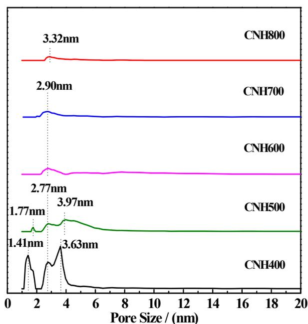
Fig. 6. Pore distribution of nanoporous  $\alpha\text{-Fe}_2\text{O}_3$ .
