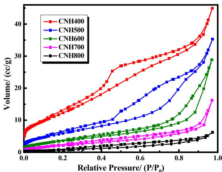
Fig. 5.  $N_2$  adsorption-desorption curves of nanoporous  $\alpha\text{-Fe}_2\text{O}_3$ .
