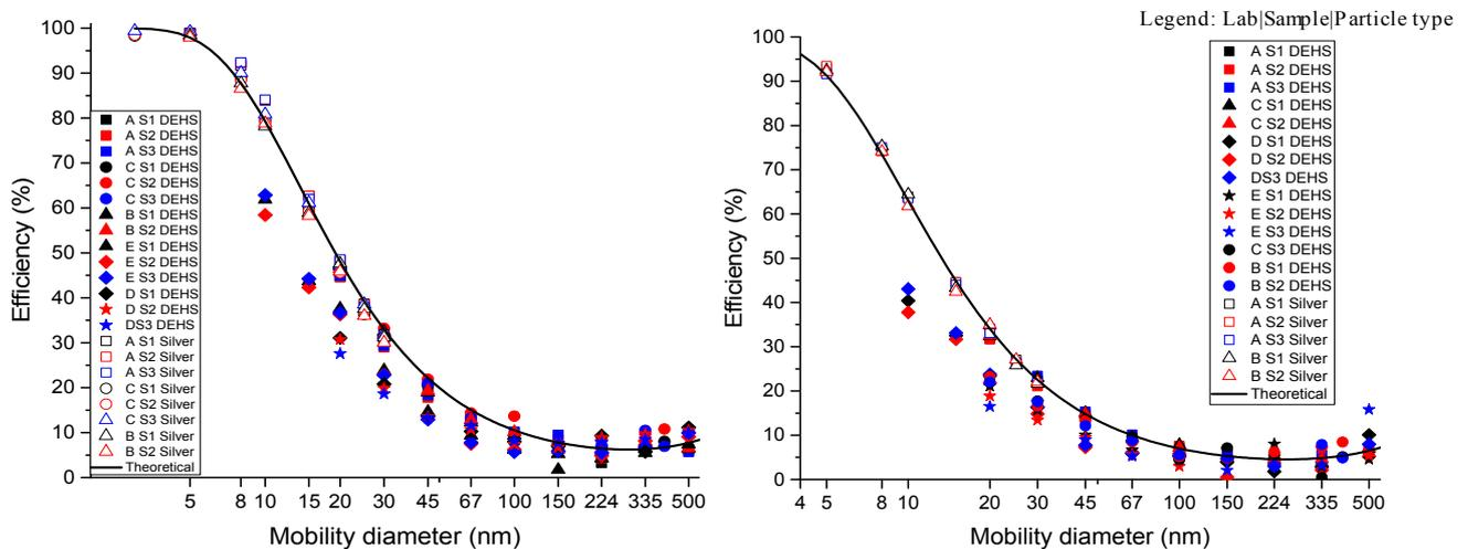
Fig. 2. Filtration efficiency test results for the wire mesh at  $5 \text{ cm s}^{-1}$  (left) and  $10 \text{ cm s}^{-1}$  (right).
