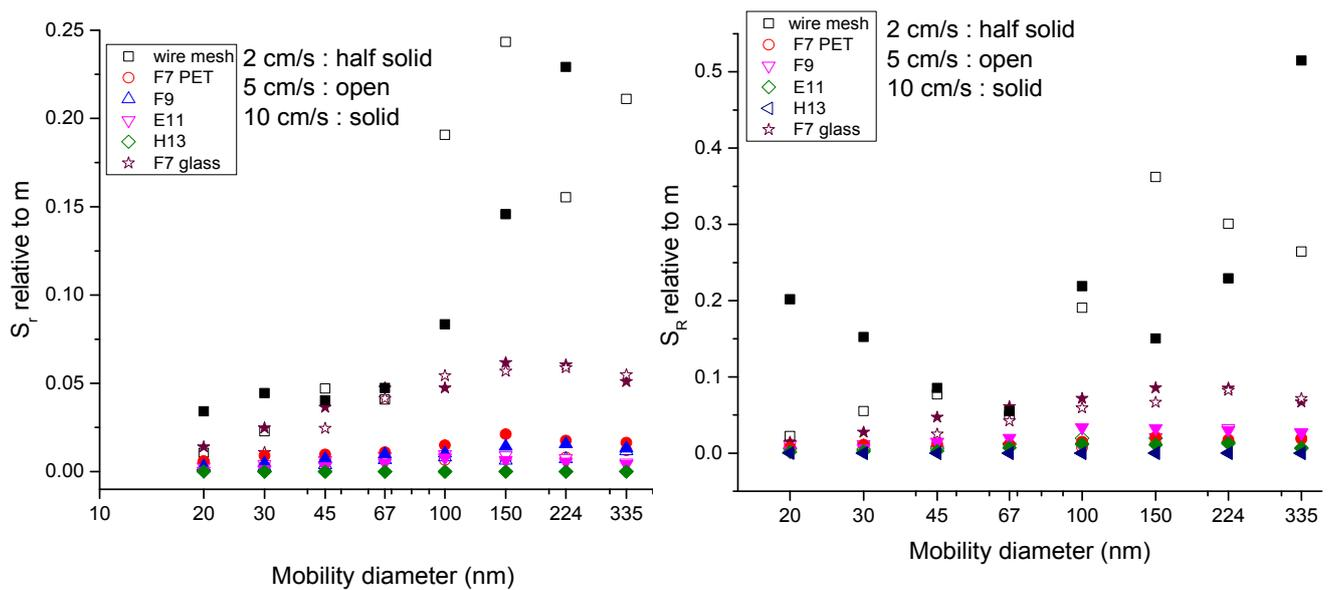
**Fig. 5.** Repeatability (left panel) and reproducibility (right panel) deviations as fractions of the average efficiency using the data of the three laboratories A, B, C and DEHS as challenging particles.
