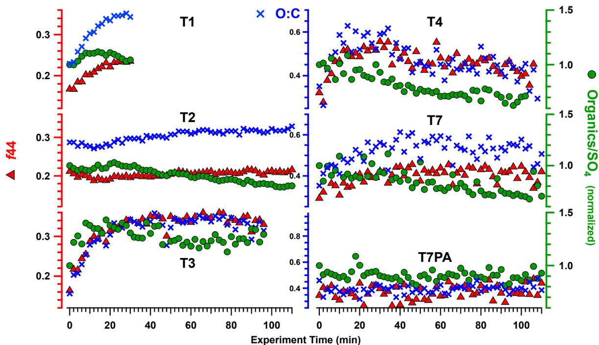
**Fig. 2.** Timelines of  $f_{44}$  (red), normalized (to  $t = 0$ ) Org/SO<sub>4</sub> (green), and O:C (blue) for T1, T2, T3, T4-1, and T7 aqueous photo-oxidations. Uncertainties (not plotted): one standard deviation equals 28% of the value, from propagation of 20% AMS quantification error through the indicated calculations. Experiment time approximates ambient oxidation time as discussed in Section 2.3.
