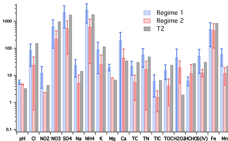
**Fig. 5.** Initial concentrations of the given cloud water constituents for given sample regimes. Units are, from left to right: Cl–Ca, HCHO, and S(IV) ( $\mu\text{N}$ ); TC–TOC (ppm); Fe and Mn ( $\mu\text{g L}^{-1}$ ). Error bars are standard deviations where data from multiple samples of the same regime were averaged. T2 consists of only one sample, so error bars are omitted.
