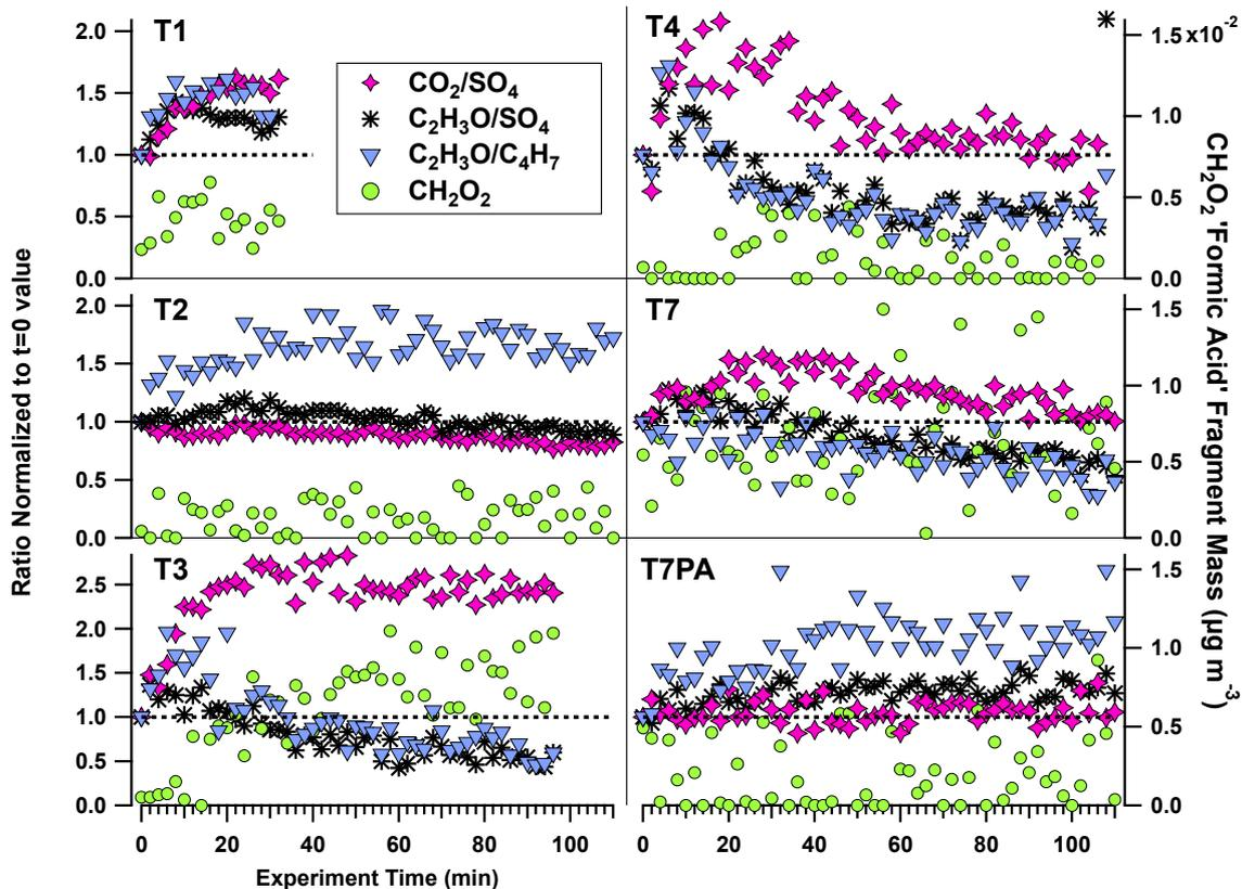
**Fig. 3.** Timelines of (left axes) fragment ratios normalized to the  $t = 0$  value and (right axes) the mass concentration of the 'formic acid' fragment for T1-4, T7, and T7PA. Uncertainties (not plotted): one standard deviation equals 28% of the value, from propagation of 20% AMS quantification error through the indicated calculations.
