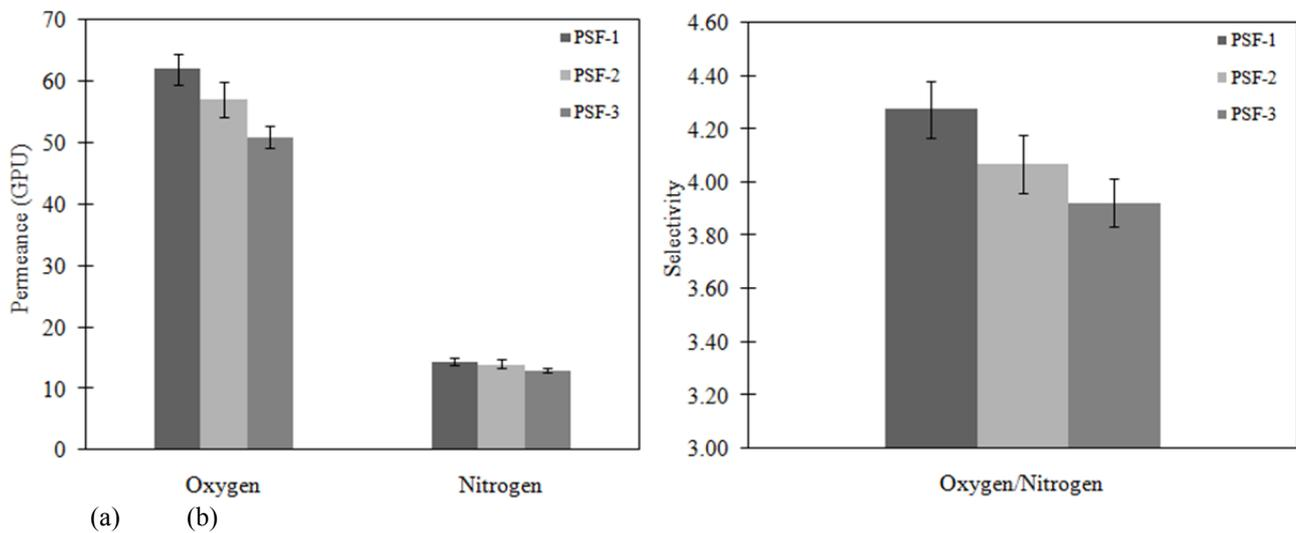
**Fig. 5.** Effect of bore fluid flow rate on (a) gas permeance and (b) selectivity.
