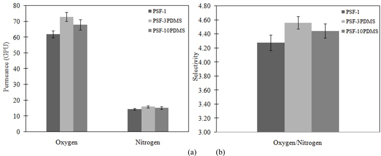
**Fig. 6.** Effect of PDMS coating on (a) gas permeance and (b) selectivity.
