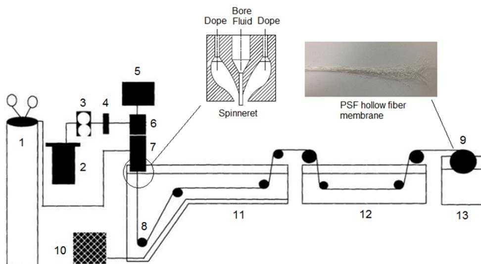
**Fig. 1.** Schematic diagram of the dry-jet wet phase inversion apparatus setup for PSF hollow fiber membrane fabrication: (1) gas cylinder; (2) dope reservoir; (3) gear pump; (4) filter (optional); (5) syringe pump; (6) spinneret; (7) force convective tube (optional); (8) roller; (9) wind-up drum; (10) refrigeration/heating unit; (11) coagulation bath; (12) washing/treatment bath and (13) wind-up bath.
