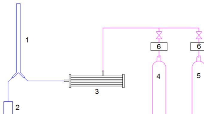
**Fig. 3.** Schematic diagram for gas permeation study: (1) soap-bubble flow meter; (2) soap container; (3) membrane module; (4) oxygen gas cylinder; (5) nitrogen gas cylinder; (6) gas pressure regulator.
