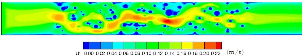
Fig. 6. Velocity magnitude contours with slip boundary conditions.
