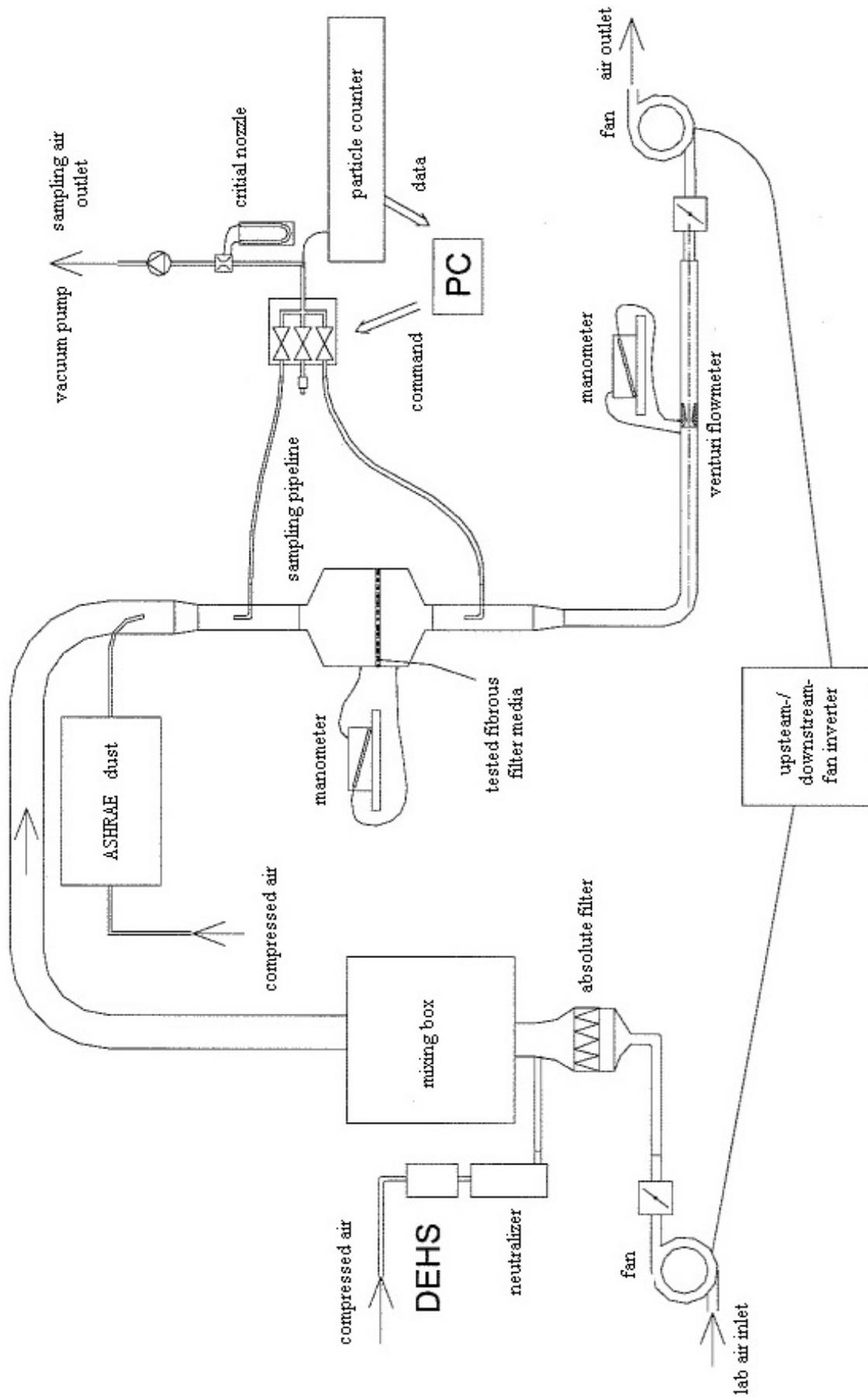
Fig. 4. Schematic diagram of the test rig.
