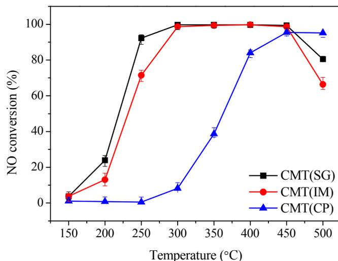
**Fig. 1.** NO conversion as a function of reaction temperature for various catalysts. Reaction conditions:  $[\text{NO}] = [\text{NH}_3] = 1000$  ppm,  $[\text{O}_2] = 3$  vol.%, balance  $\text{N}_2$  and GHSV =  $90,000 \text{ h}^{-1}$ .
