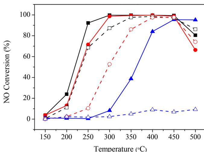
**Fig. 2.** Effect of  $\text{H}_2\text{O}$  on NO conversion over various catalysts. ( $\blacksquare$ ) CMT(SG), ( $\bullet$ ) CMT(IM), ( $\blacktriangle$ ) CMT(CP). Reaction conditions:  $[\text{NO}] = [\text{NH}_3] = 1000$  ppm,  $[\text{O}_2] = 3$  vol.%,  $[\text{H}_2\text{O}] = 10\%$  ( $\square$ ,  $\circ$ ,  $\triangle$ ), balance  $\text{N}_2$  and GHSV =  $90,000 \text{ h}^{-1}$ .
