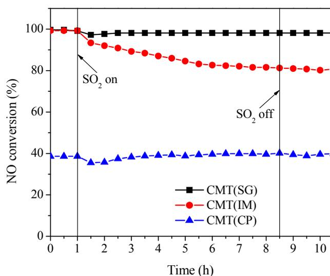
**Fig. 3.** Effect of  $\text{SO}_2$  on NO conversion over various catalysts at  $350^\circ\text{C}$ . Reaction conditions:  $[\text{NO}] = [\text{NH}_3] = 1000$  ppm,  $[\text{O}_2] = 3$  vol.%,  $[\text{SO}_2] = 1000$  ppm, balance  $\text{N}_2$  and GHSV =  $90,000$   $\text{h}^{-1}$ .
