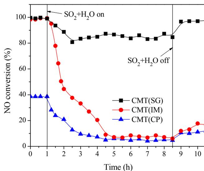
**Fig. 4.** Effect of  $\text{H}_2\text{O}$  and  $\text{SO}_2$  on NO conversion over various catalysts at  $350^\circ\text{C}$ . Reaction conditions:  $[\text{NO}] = [\text{NH}_3] = 1000$  ppm,  $[\text{O}_2] = 3$  vol.%,  $[\text{H}_2\text{O}] = 10\%$ ,  $[\text{SO}_2] = 1000$  ppm, balance  $\text{N}_2$  and GHSV =  $90,000$   $\text{h}^{-1}$ .
