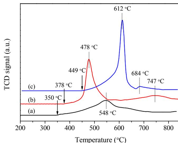
**Fig. 8.** H<sub>2</sub>-TPR profiles of (a) CMT(SG), (b) CMT(IM) and (c) CMT(CP).
