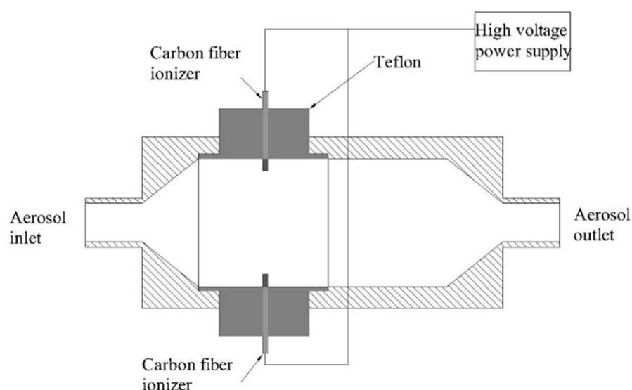
**Fig. 8.** Schematic diagram of the unipolar charger developed by Han *et al.* (2008).
