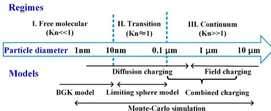
Fig. 1. The scale comparison of charging models.
