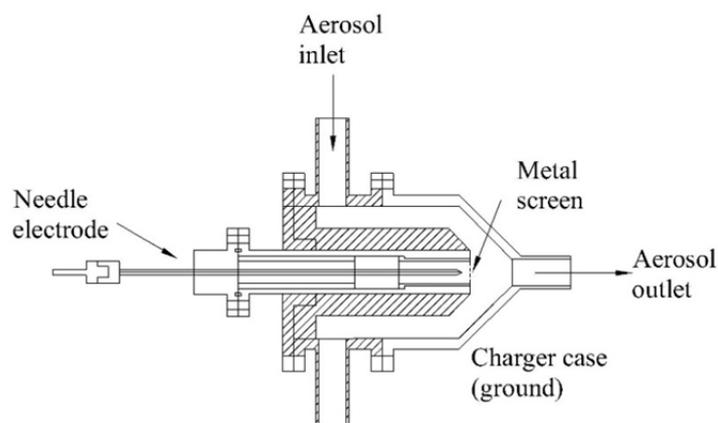
**Fig. 10.** Schematic diagram of the DC-corona based charger developed by Li and Chen (2011b).
