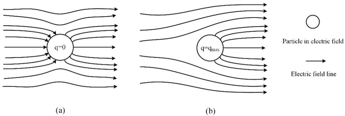
**Fig. 2.** Electric field line around a particle (a) an uncharged particle (b) a particle with saturation charge.
