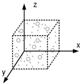
**Fig. 4.** Schematic representation of the Monte-Carlo simulation volume (Biskos *et al.*, 2004).
