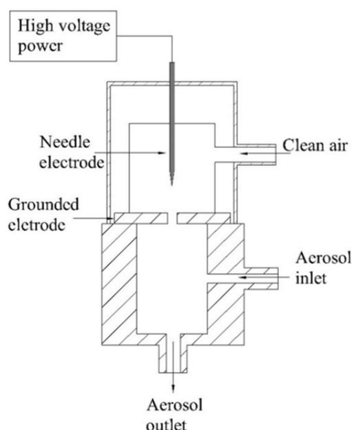
**Fig. 9.** Schematic diagram of the small mixing-type unipolar charger developed by Kimoto (2010).
