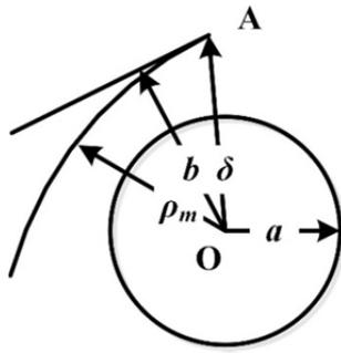
**Fig. 3.** Motion of ions inside the limiting sphere (Fuchs, 1963).
