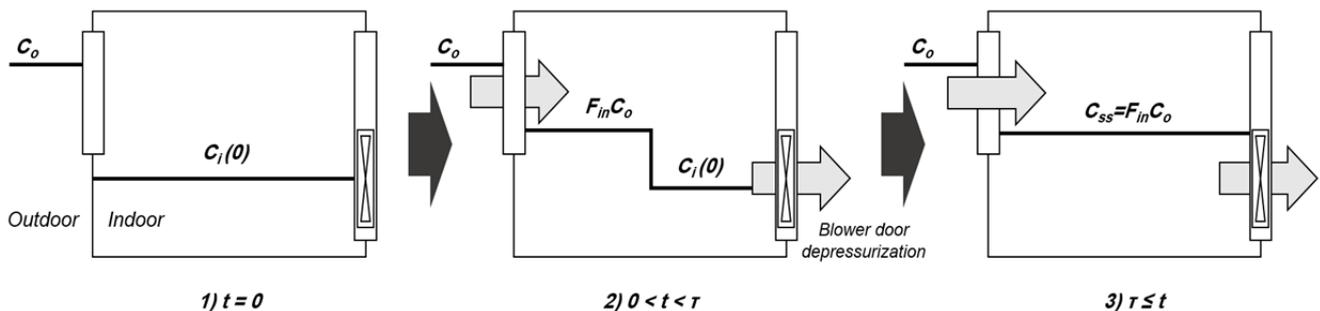
**Fig. 1.** Schematic diagram of the infiltration test procedure.
