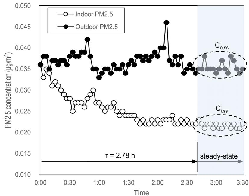
**Fig. 3.** An example of ambient and indoor PM<sub>2.5</sub> concentration profile during the infiltration test (Unit G).
