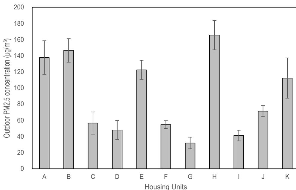
**Fig. 2.** Average and standard deviation of ambient  $PM_{2.5}$  concentration on the day of testing for each unit.
