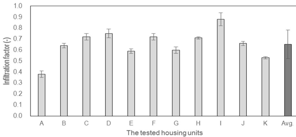
**Fig. 4.** PM<sub>2.5</sub> infiltration factors in test housing units.
