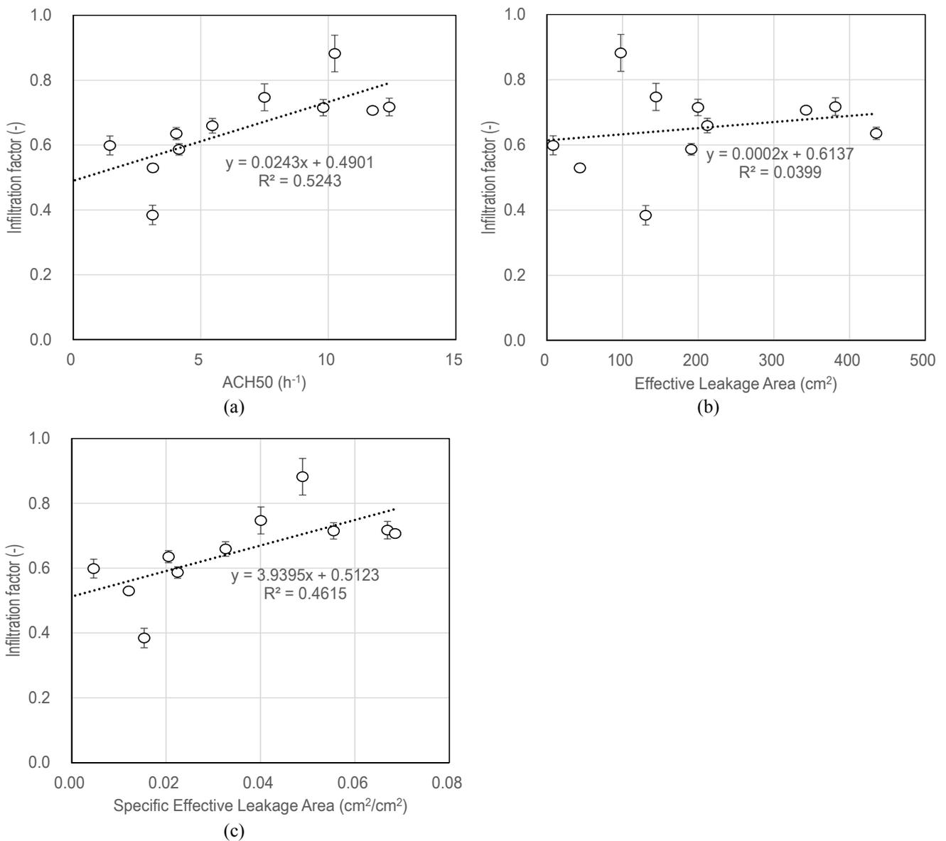
**Fig. 5.** Relationship of infiltration factors to airtightness test results: a) ACH<sub>50</sub>; b) Effective leakage area (ELA); c) Specific effective leakage area (sELA).
