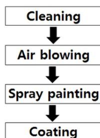
**Fig. 1.** A process diagram of the spray painting with powder coatings.
