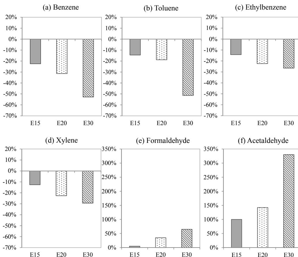
**Fig. 3.** Emission change (%) of the air toxics for the ethanol blends (E15, E20, and E30) compared with that of RF; (a) benzene, (b) toluene, (c) ethylbenzene, (d) xylene, (e) formaldehyde, and (f) acetaldehyde.
