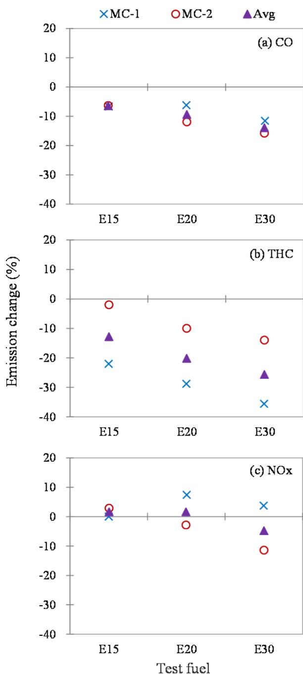
**Fig. 1.** Emission change (%) of criteria air pollutant of the ethanol-gasoline blends compared with those of the commercial fuel (RF); (a) CO, (b) THC, and (c) NO<sub>x</sub>.
