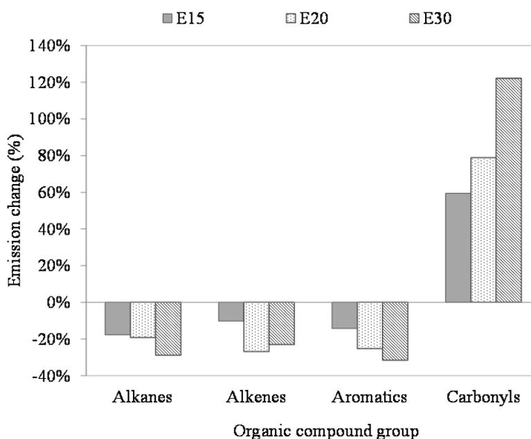
**Fig. 2.** Emission change (%) of organic group of the ethanol-gasoline blends compared with those of the commercial fuel (RF).**Table 4.** Emissions ( $\text{mg km}^{-1}$ ) of air toxics from the four-stroke motorcycle for the ethanol-gasoline blends.
