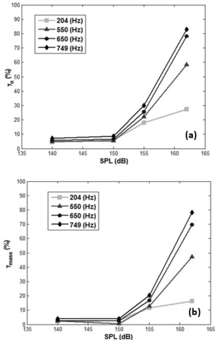
**Fig. 8.** Variation of (a) acoustic coagulation and precipitation efficiency ( $\gamma_n$ ) and (b) acoustic precipitation efficiency ( $\gamma_{\text{mass}}$ ), against SPL in the different frequencies after 10 min.
