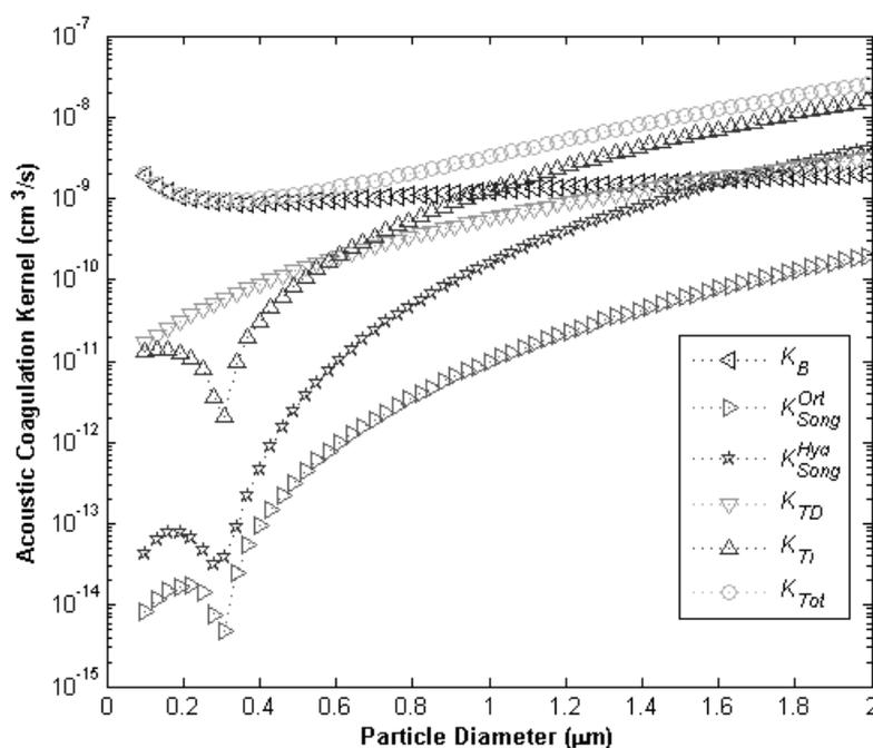
**Fig. 2.** Evolution of acoustic coagulation kernels (logarithmic scale) of a particle with ( $0.3 \mu\text{m}$ ) with particles in the range of ( $0.1\text{--}2 \mu\text{m}$ ) at 162 dB and 749 Hz ( $K_B$ -Brownian Kernel,  $K^{\text{Ort}}$ - Song Orthokinetic Kernel,  $K^{\text{Hya}}$ -Song Hydrodynamic Kernel,  $K^{\text{TD}}$ -Turbulent Diffusional Kernel,  $K^{\text{TI}}$ -Turbulent Inertial Kernel and  $K^{\text{Tot}}$ -Total Kernel).
