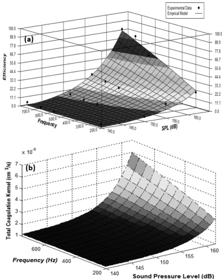
**Fig. 9.** (a) Comparison of experimental data and predicted value by the empirical model, (b) Evolution of acoustic coagulation kernels (particle-1 (0.3  $\mu\text{m}$ ) and particle-2 (0.8  $\mu\text{m}$ )) with respect to the frequency (204–749 Hz) and sound pressure level (140–162 dB).
