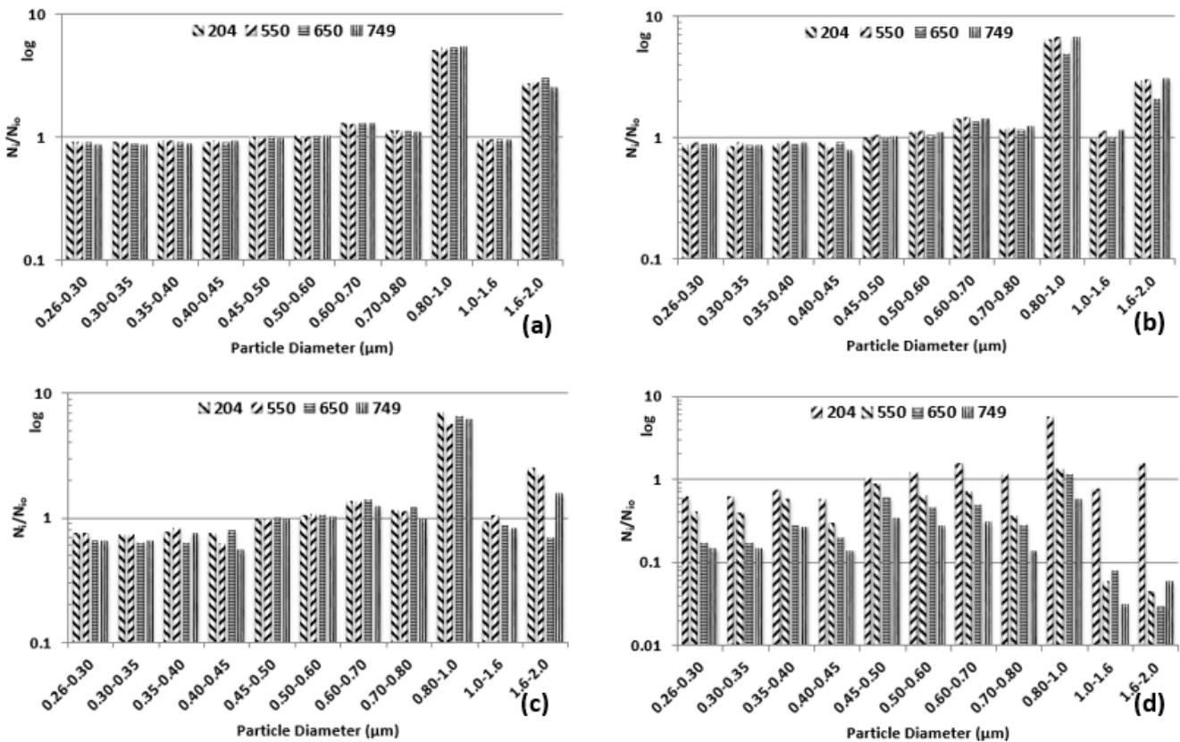
Fig. 7. Evolution of  $(N_i/N_{i0})$  against Frequency (Hz) and after 10 min at (a) 140 dB, (b) 150 dB, (c) 155 dB and (d) 162 dB.
