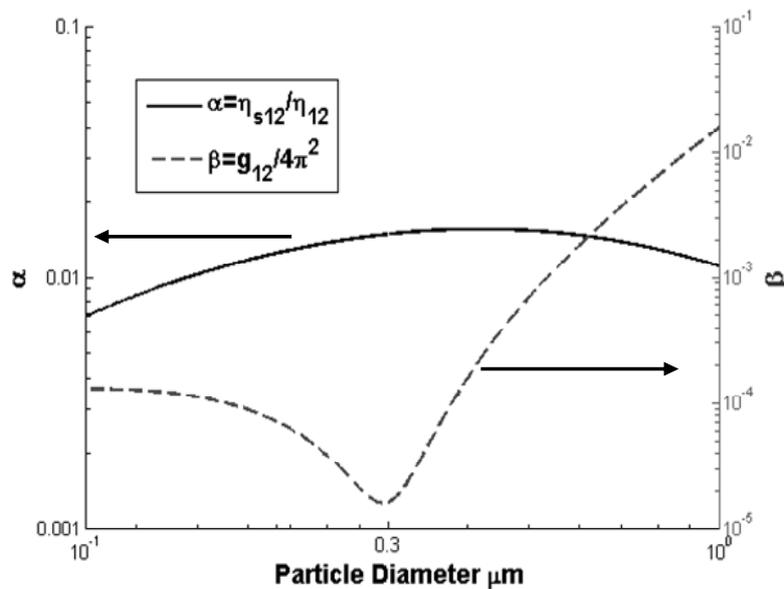
**Fig. 1.** The calculated collision efficiency ( $\alpha$ ) and hydrodynamic interaction factor ( $\beta$ ). The data were calculated for the collision between a particle of 0.3  $\mu\text{m}$  and a particle of 0.1–1  $\mu\text{m}$ .
