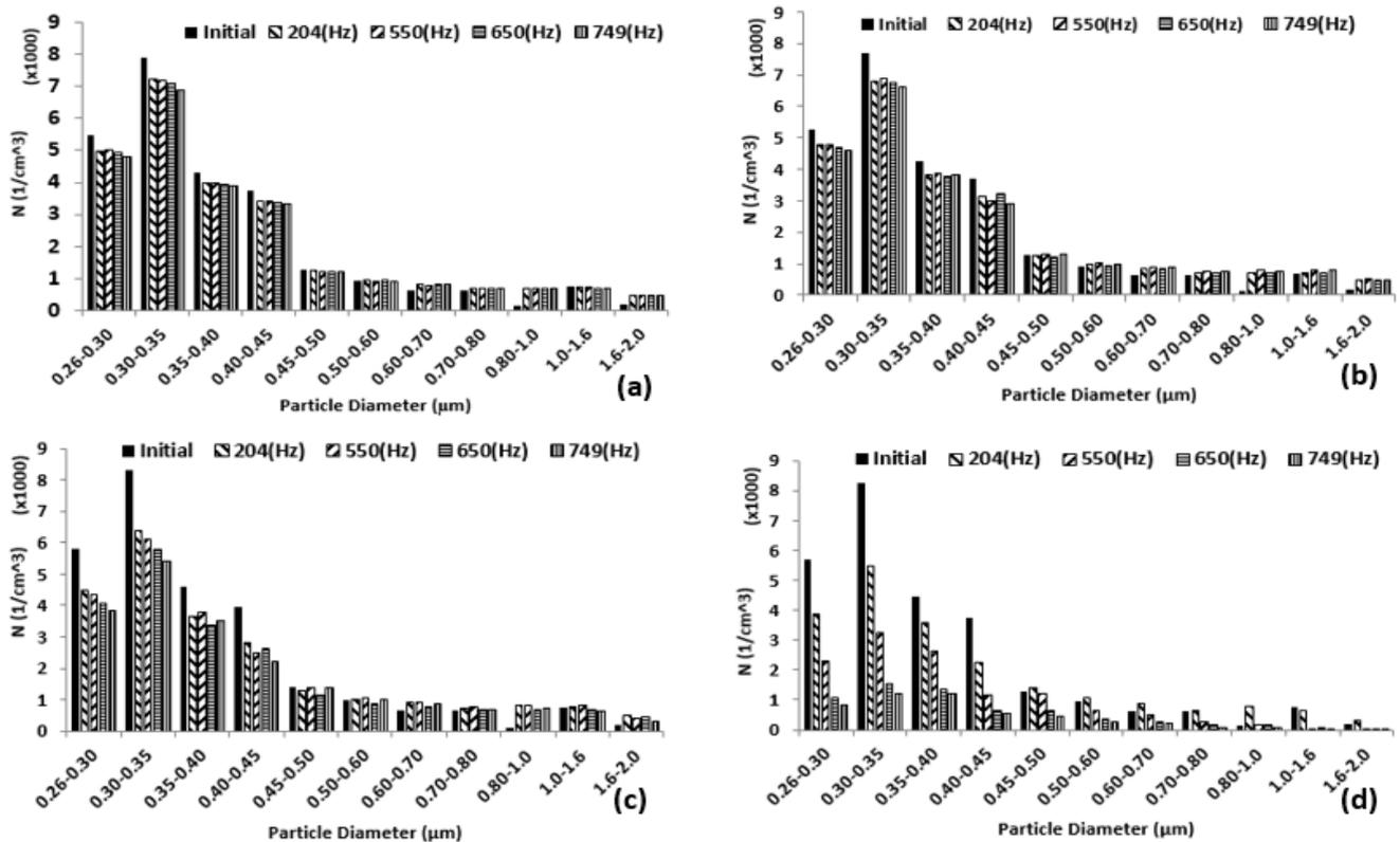
**Fig. 6.** PSD evolution at different frequencies of acoustic radiation and after 10 min at (a) 140 dB, (b) 150 dB, (c) 155 dB and (d) 162 dB.
