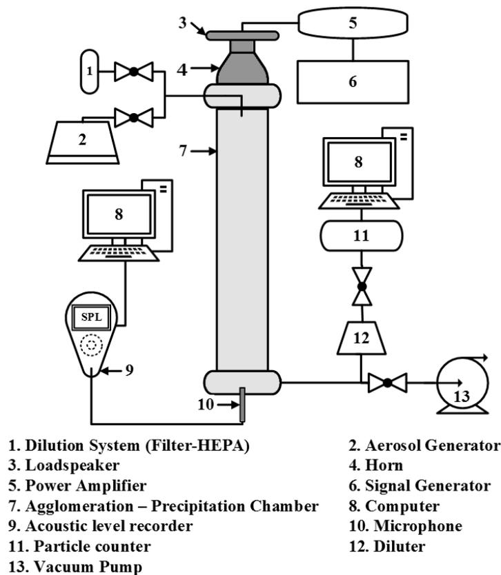
Fig 4. A schematic view of Experimental Setup.
