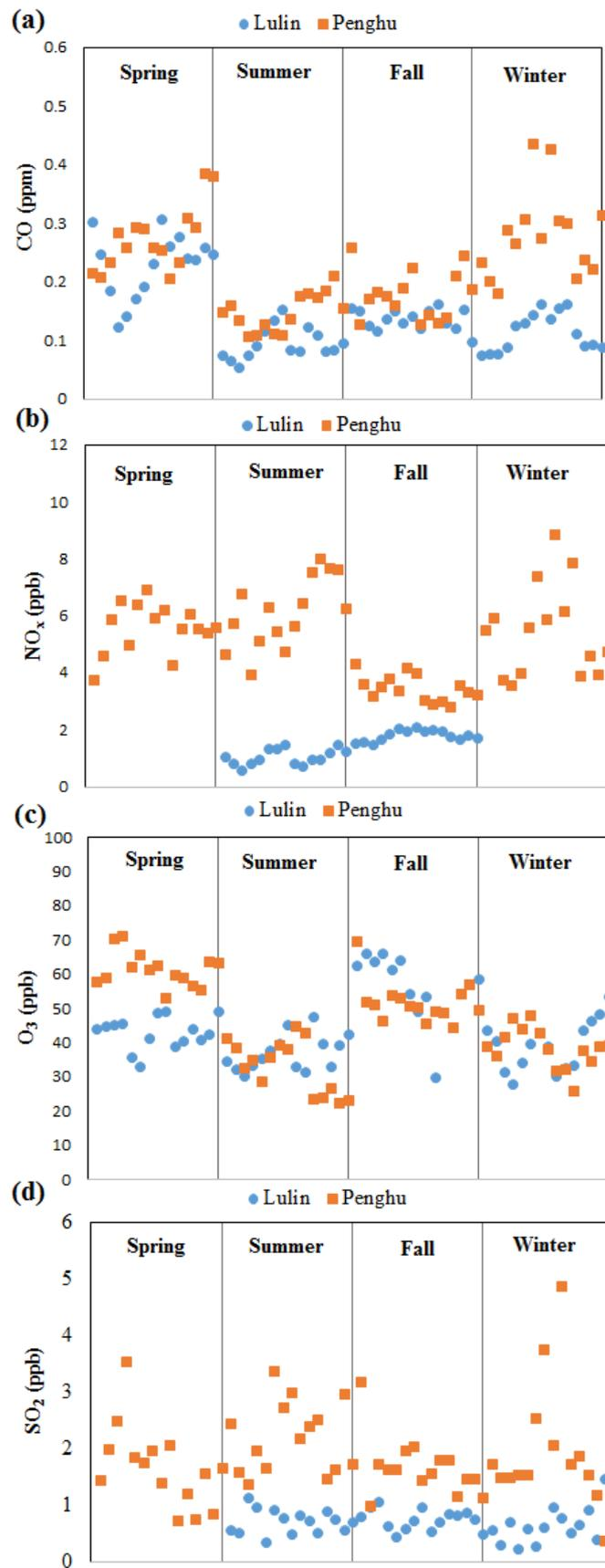
**Fig. 5.** Seasonal variation of air pollutants at the two remote sites for (a) carbon monoxide, (b) nitrogen dioxide, (c) ozone, and (d) sulfur dioxide.
