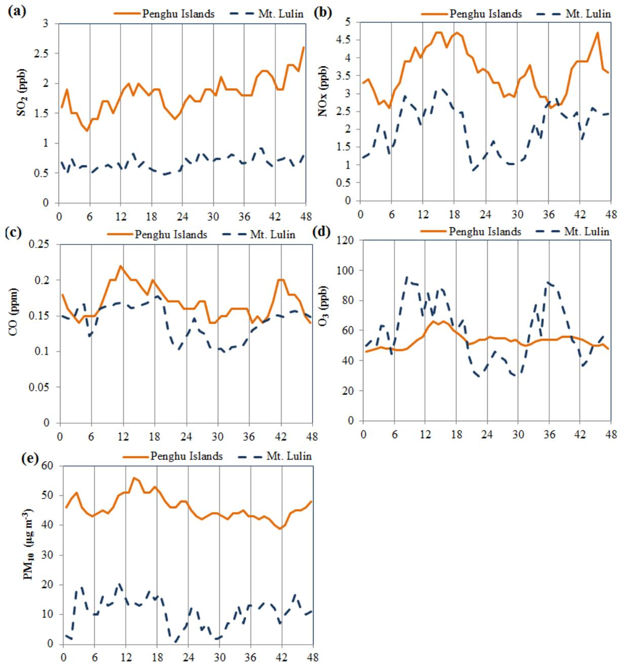
**Fig. 4.** Hourly variation of air pollutant measured at two remote sites, the Mt. Lulin and the Penghu Islands for (a) sulfur dioxide, (b) nitrogen oxides, (c) carbon monoxide, (d) ozone, (e) PM<sub>10</sub>. The solid line (—) represents the Penghu Islands and the dash line (- -) represents the Mt. Lulin.
