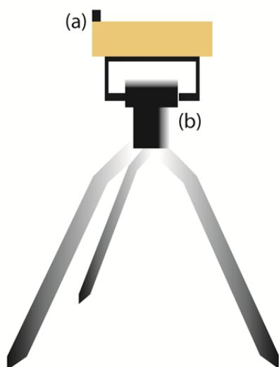
**Fig. 1.** GLOBE Sun Photometer setup: (a) photometer and (b) two servos with pan and tilt mount. Not shown: small rack to hold the ozone, temperature, and pressure sensors along with Raspberry Pi and wiring.
