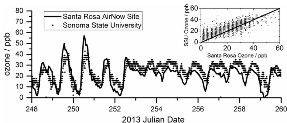
**Fig. 4.** Comparison of ozone measurements from this study (dots) with an AirNow site, 7.4 mi NNW as a function of time (main graph) and versus each other (inset, with 1:1 line drawn).
