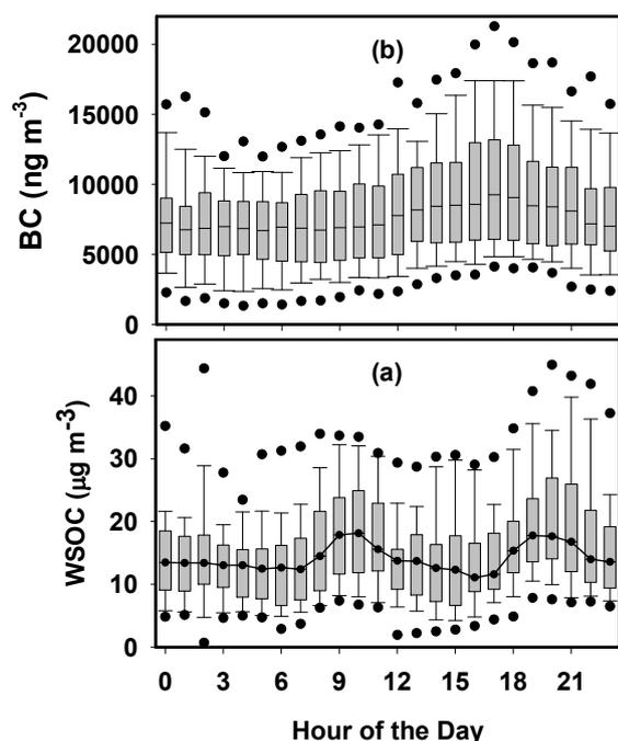
**Fig. 3.** Comparison of diurnal variability in (a) WSOC (can be both primary and secondary particle) and (b) BC (primary particle only) during the study period suggests that a considerable fraction of WSOC is secondary. Each bin of this whisker plot represents  $\sim 400$  data points.
