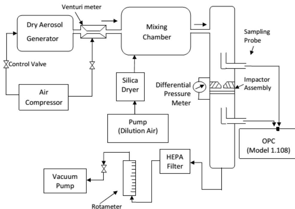
Fig. 1. Experimental setup for impactor characterization in the laboratory.
