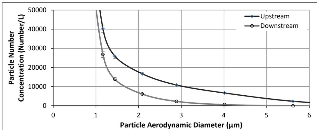
Fig. 3. Size distribution variation from a representative test.
