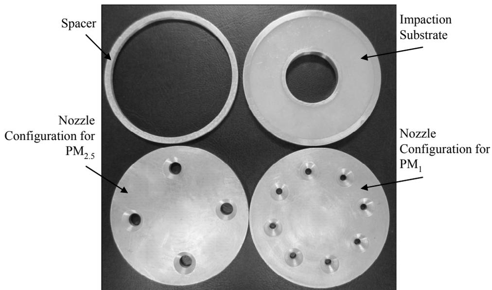
Fig. 2. Components of the optimum PM<sub>1</sub>/PM<sub>2.5</sub> impactor assembly.
