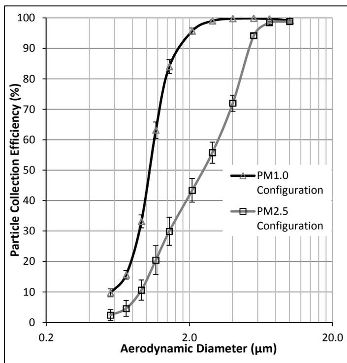
Fig. 4. Collection efficiency curves for optimum PM<sub>1</sub>/PM<sub>2.5</sub> impactors.
