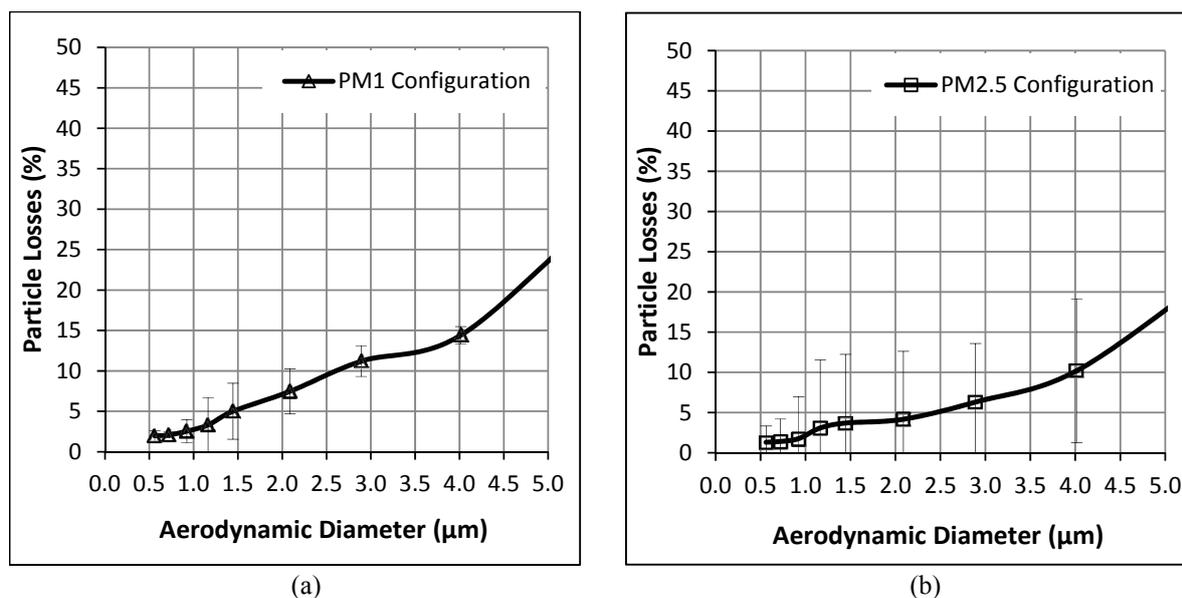
Fig. 5. Overall particle losses in the impactor for (a) PM<sub>1</sub> and (b) PM<sub>2.5</sub> configuration, respectively.
