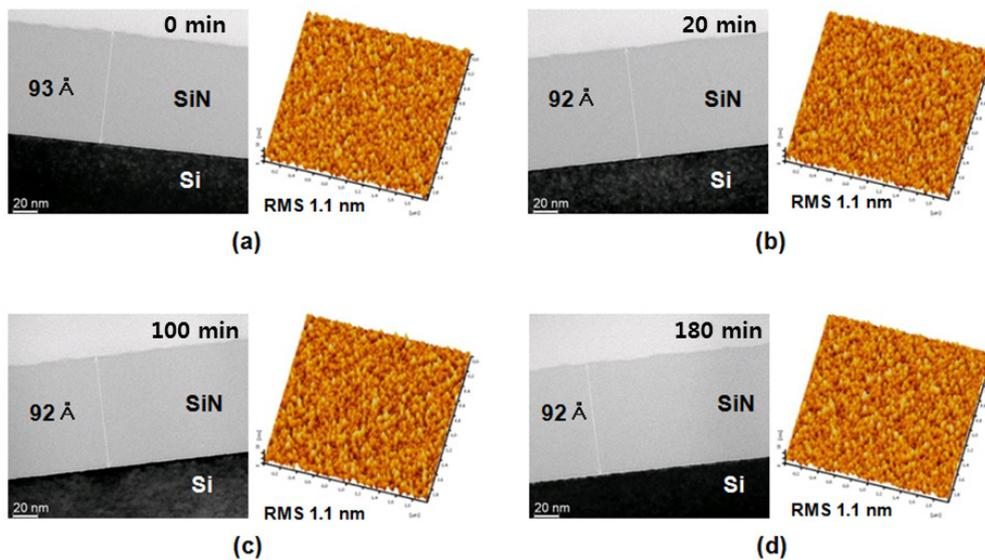
**Fig. 8.** Variation of SiN layer thickness and morphology depending on storage times of 0 (a), 20 (b), 100 (c) and 180 (d) minutes in the contaminated FOUP.
