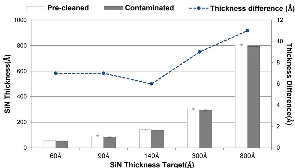
**Fig. 4.** Thickness of SiN deposited film layer of wafers stored in the pre-cleaned (□) and the contaminated (■) FOUPs, and thickness difference ratio (---●---) of SiN layers stored in the contaminated FOUP.
