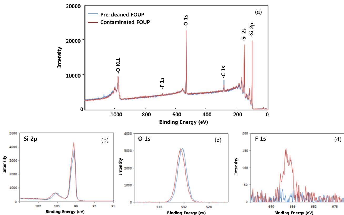
**Fig. 5.** XPS spectra of clean silicon wafers stored in each pre-cleaned FOUP and contaminated FOUP for an hour (a), and magnified spectrums of silicon (b), oxygen (c) and fluoride (d) detection.
