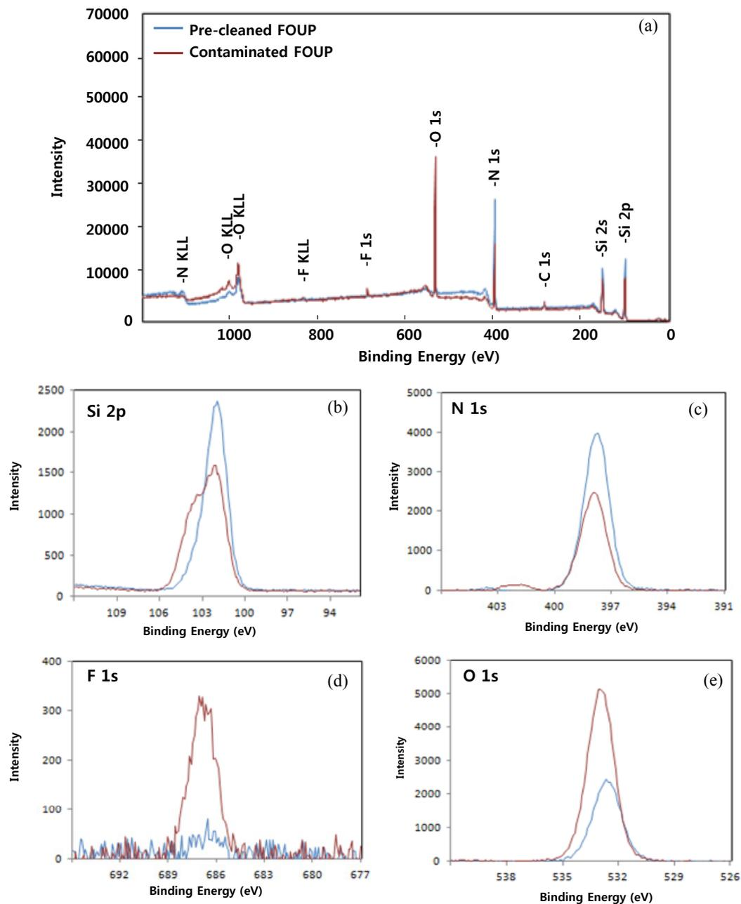
**Fig. 6.** XPS spectra of SiN as-deposited wafers stored in each pre-cleaned FOUP and contaminated FOUP for an hour (a), and magnified spectra of silicon (b), nitrogen (c), fluoride (d) and oxygen (d) detection.
