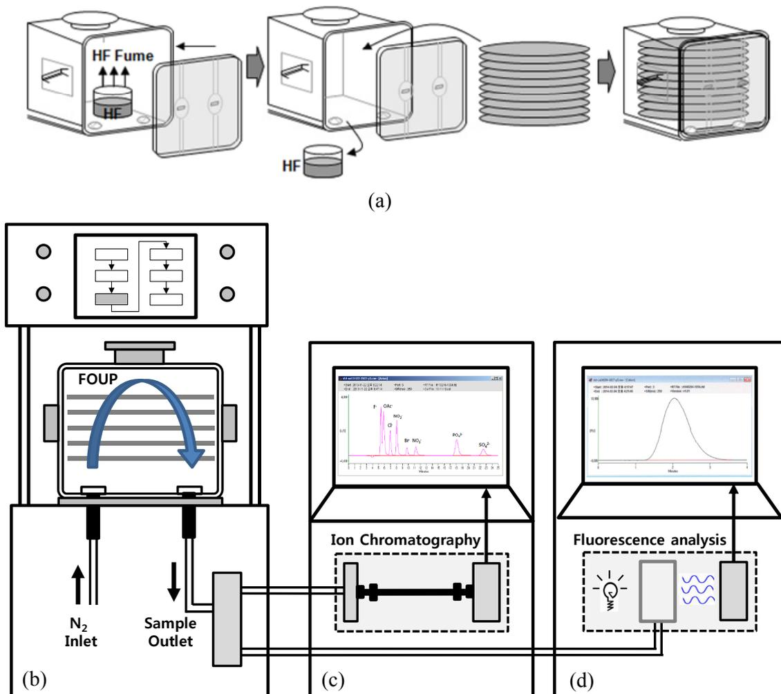
**Fig. 1.** Schematic diagram for artificial contamination of the inside of FOUP (a), and automated sampling system (b) connected with the analyzers for ion chromatography (c) and fluorescence analysis (d).
