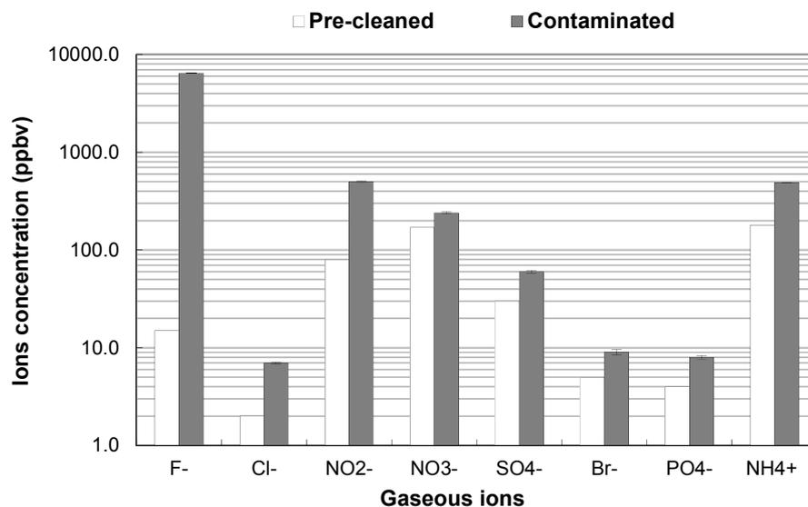
Fig. 3. Concentration of gaseous ions detected in the pre-cleaned (□) and contaminated (■) FOUP.
