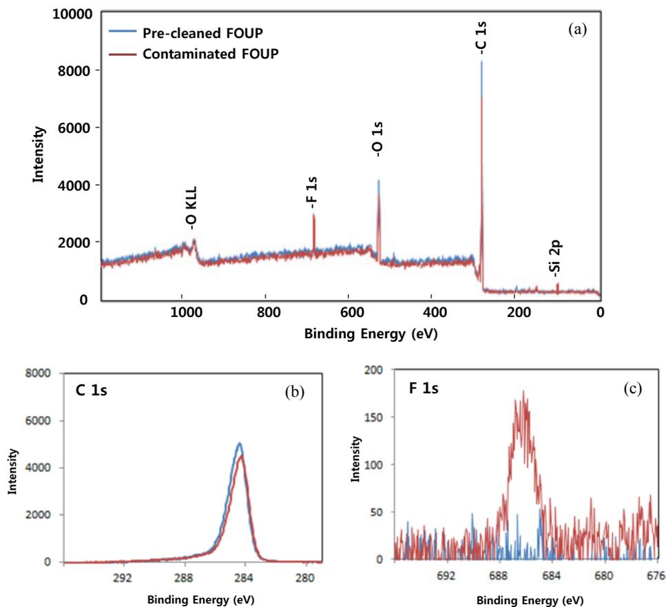
**Fig. 7.** XPS spectra of inner surface of pre-cleaned FOUP and contaminated FOUP (a), and magnified spectra of carbon (b) and fluoride detection.
