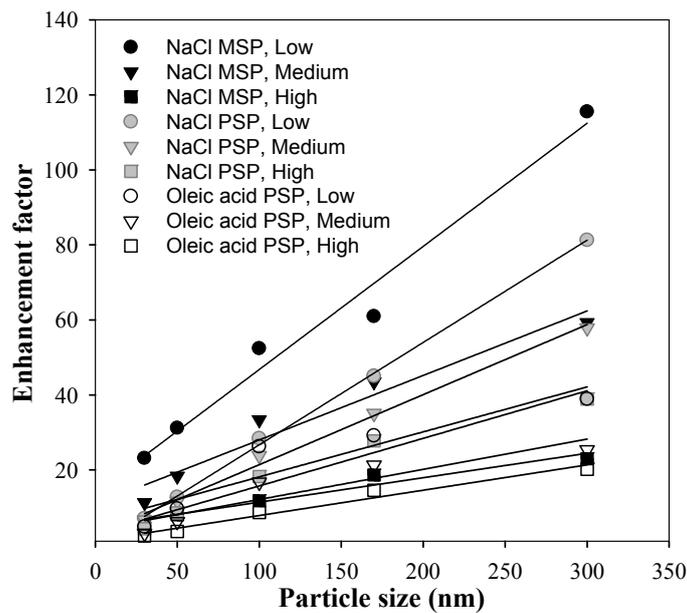
**Fig. 7.** The relationship between EF and particle size (diameter) under various freestream air velocities (Low, Medium and High).
