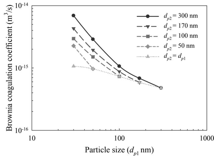
**Fig. 3.** Brownian coagulation coefficient  $K_{1,2}$  for coagulation of particles of diameters  $d_{p1}$  and  $d_{p2}$ .
