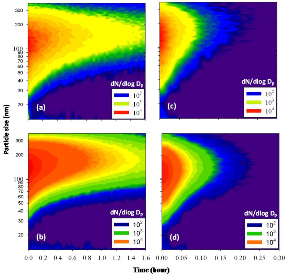
**Fig. 4.** The time profile of PSP size distribution and concentration under low freestream air velocity (a)(b) NAI off; (c)(d) NAI on; (a)(c) NaCl PSP; (b)(d) Oleic acid PSP.
