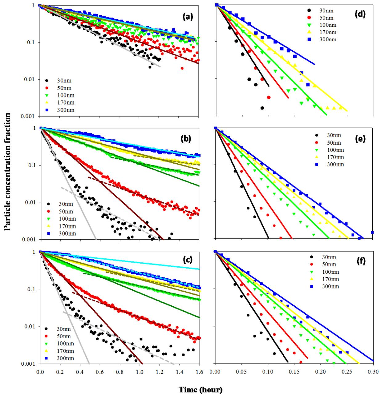
**Fig. 5.** The time profile of (a)(d)NaCl MSP; (b)(e) NaCl PSP; (c)(f) Oleic acid PSP number concentrations under low freestream air velocity (a)(b)(c) NAI off; (d)(e)(f) NAI on; the short dash fitting curves in (b) and (c) have similar slopes to the corresponding fitting curves in (a), indicating that the decay rate is similar.
