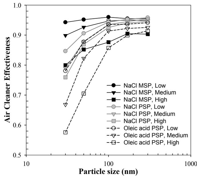
**Fig. 8.** The relationship between  $ACE$  and particle size under different freestream air velocities (Low, Medium and High).
