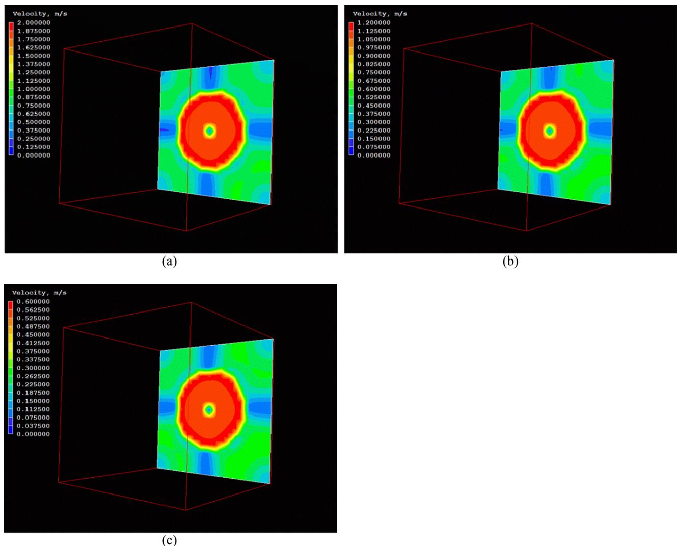
**Fig. 2.** Air velocity patterns in the chamber (a) high freestream air velocity (b) medium freestream air velocity (c) low freestream air velocity.
