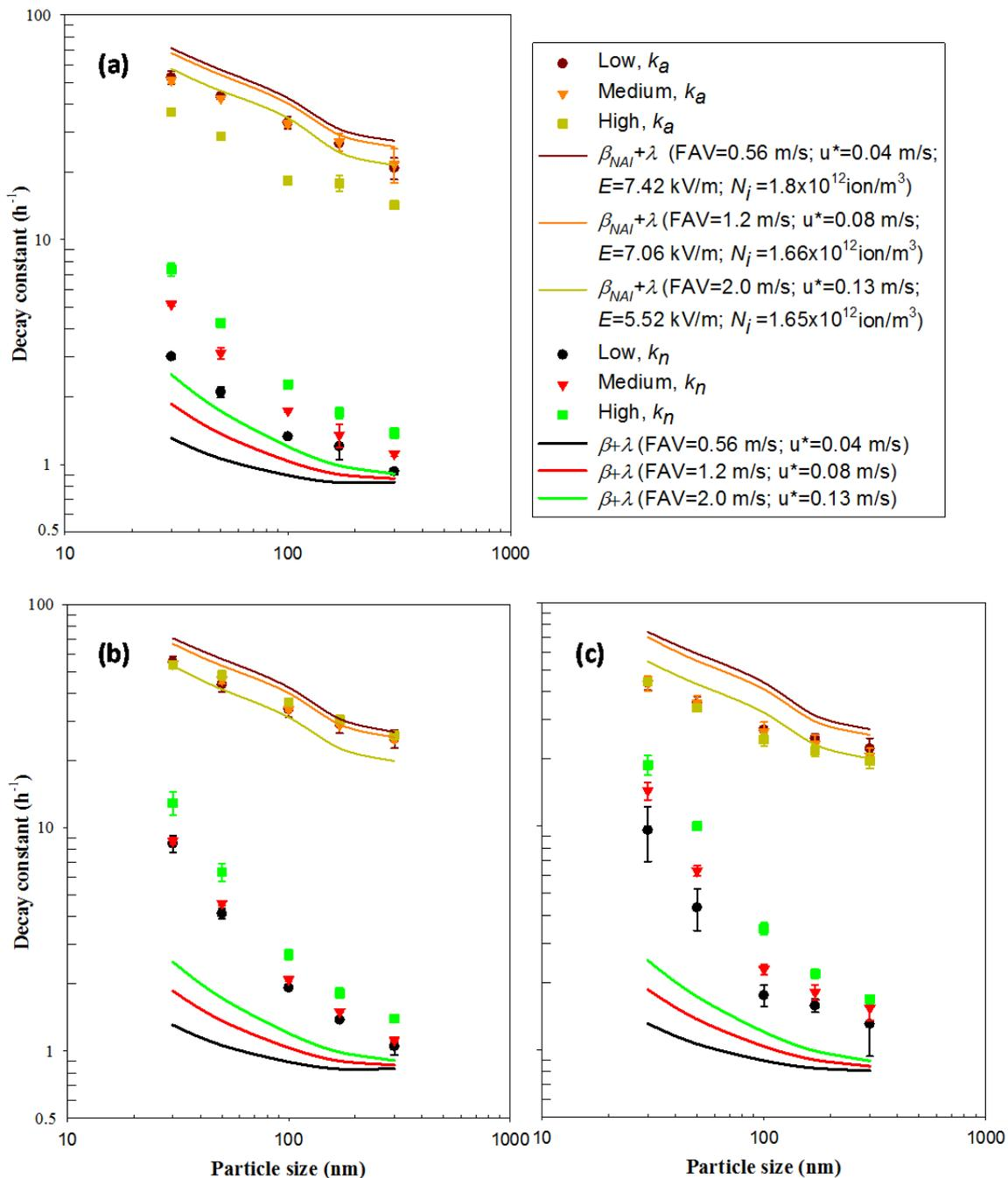
**Fig. 6.** The relationship between decay constants and particle sizes under various friction velocities (a) NaCl MSP (b) NaCl PSP (c) Oleic acid PSP. FAV: freestream air velocity.
