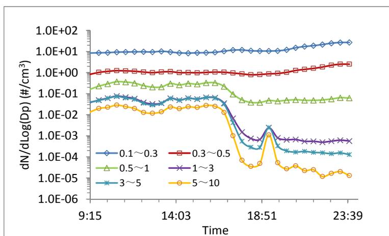
**Fig. 2.** Diurnal variation of size fractionated particle number concentration in the Gallery of Ceramics hall on October 1<sup>st</sup>.
