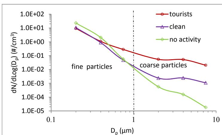
**Fig. 5.** Particle number size distributions during the open time, cleanup time and night in the museum.
