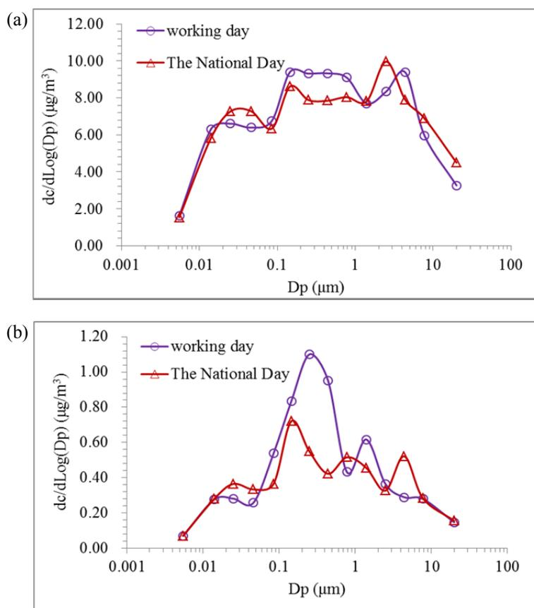
**Fig. 9.** Size-fractionated elemental carbon (a) and organic carbon (b) concentrations on working day and the National Day.
