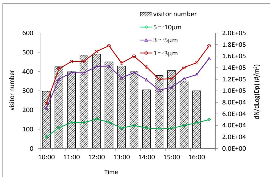
**Fig. 4.** Visitor flow rate and particle number concentration in different time periods in the Ancient Chinese Ceramics hall on October 1<sup>st</sup>.
