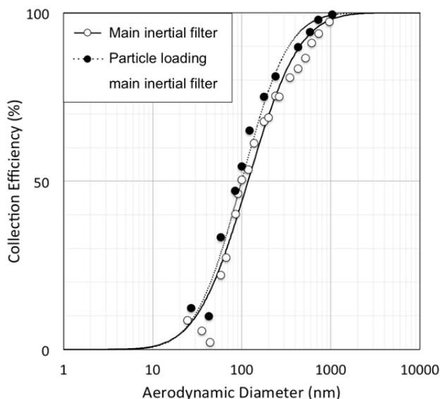
**Fig. 8.** Comparison of collection efficiency of the main inertial filter before and after the particle loading of 0.1 mg.
