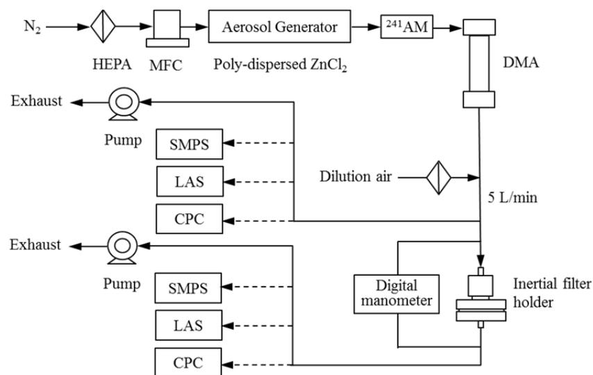
**Fig. 3.** An experimental setup for the inertial filter performance test.
