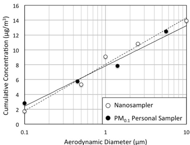
**Fig. 9.** Comparison of aerosol particle cumulative concentrations obtained by  $PM_{0.1}$  personal sampler with Nanosampler for ambient aerosol sampling.
