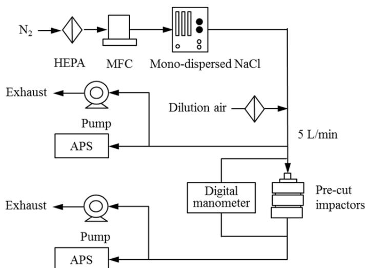
**Fig. 4.** An experimental setup for the pre-cut impactors performance test.
