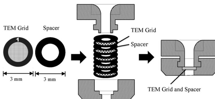
**Fig. 1.** Schematic of the main inertial filter.
