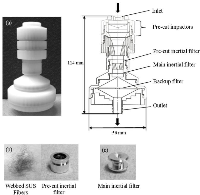
**Fig. 2.**  $PM_{0.1}$  personal sampler inlet and inertial filters used: (a) an outside picture and structure of  $PM_{0.1}$  personal sampler inlet, (b) the pre-cut inertial filter and stainless steel (SUS) fibers used, and (c) the main inertial filter (layered mesh geometry).
