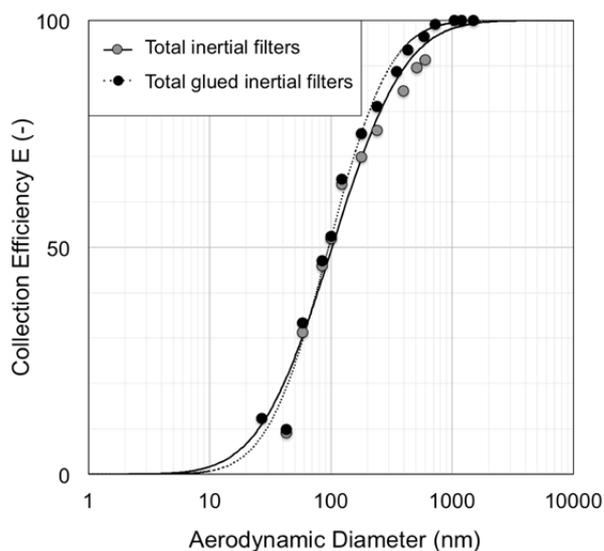
**Fig. 7.** Effect of glue coating on the total collection efficiency of the pre-cut and main inertial filters.
