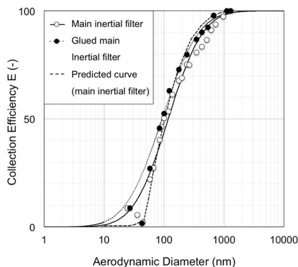
**Fig. 6.** Effect of glue coating on TEM grids on the collection efficiency of the main inertial filter.
