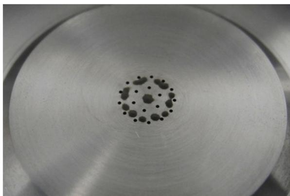
**Fig. 3.** Picture of jet-plate surface deposits on DLPI stage 4 ( $D_{50\%} = 0.155 \mu\text{m}$ ).
