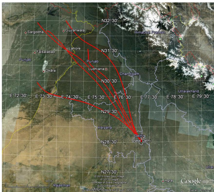
Fig. 6. Back-trajectories at a site in Delhi for few days of  $PM_{2.5} > 300 \mu g/m^3$  during 2007–2009 at starting time of 0000 UTC and altitude of 500 m AGL calculated using NOAA HYSPLIT model with meteorological data set-GDAS, total run time-24 hrs and location ( $28.54^\circ 77.188^\circ$ ). The origin of the trajectories is marked with a dot and the trajectories are marked with red color.
