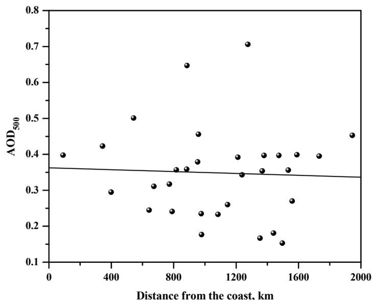
**Fig. 16.** Variation of AOD at 500 nm as a function of distance from the coast over the BoB considering, Chennai (13.1°N, 80.2°E) as the coast. The straight lines represent the least squares fit following Eq. (7).
