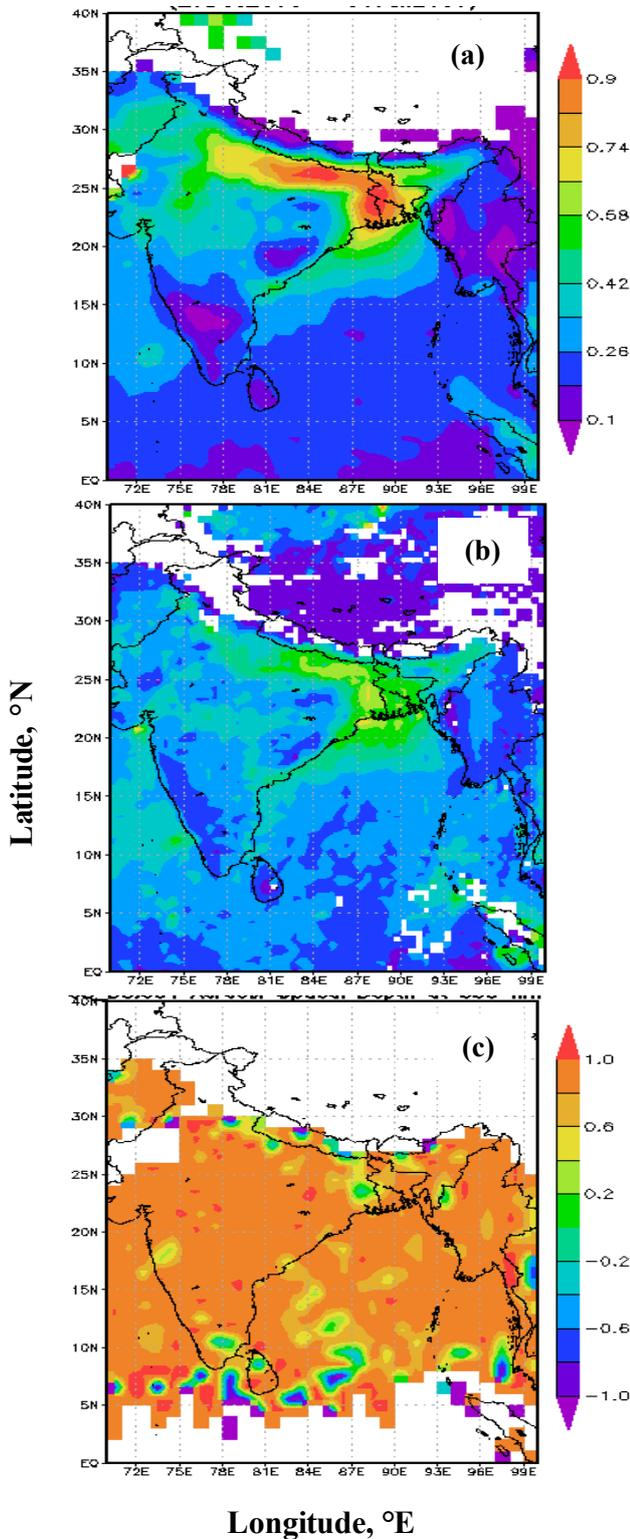
**Fig. 9.** Monthly mean spatial distribution of AOD over BoB retrieved from (a) MODIS (b) MISR and (c) spatial correlation between MODIS and MISR derived AOD for the study period. The colored scale is common for both AODs retrieved from MODIS and MISR.
