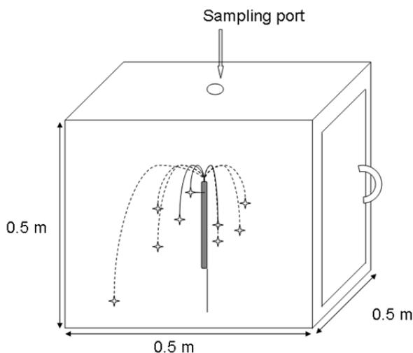
Fig. 1. Experimental chamber.
