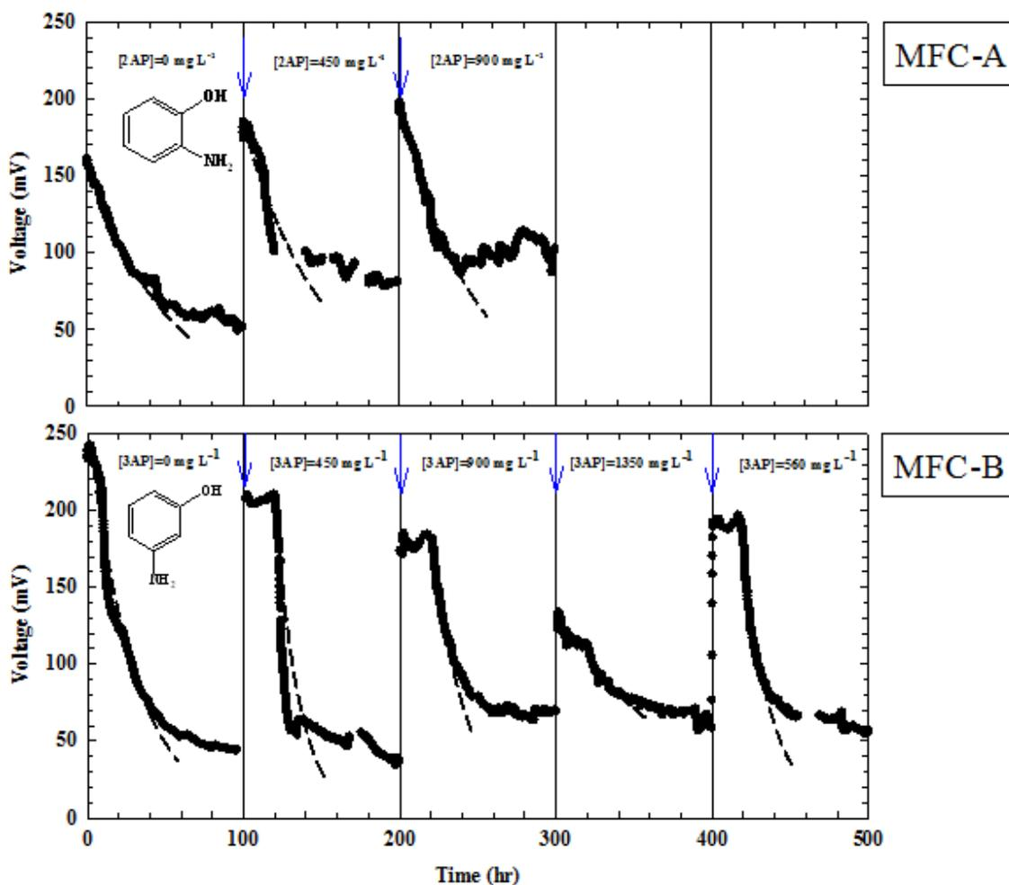
**Fig. 2.** Time course of bioelectricity generation of *Proteus hauseri* ZMd44 in MFC-A and MFC-B supplemented with various concentrations of 2-AP, 3-AP (external resistance = 1 K $\Omega$ ). Dashed curves denoted model prediction of output voltage profiles (raw data after Chen *et al.* (2011a)).
