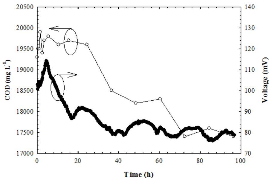
**Fig. 1.** Time courses of COD degradation and cell voltage in *Acinetobacter* sp. x72-dominated MFC using 0.2x LB medium as energy source (external resistance 1 K $\Omega$ ). Initial decay rate constant for bioelectricity generation and initial decay rate constant of COD degradation were ca. 0.45 and 0.0015 h<sup>-1</sup>, respectively.
