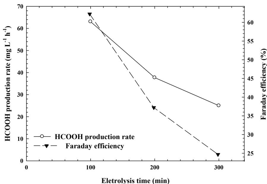
**Fig. 6.** Variations in the formic acid production rate and the Faraday efficiency with electrolysis time in CO<sub>2</sub> electrolysis process.
