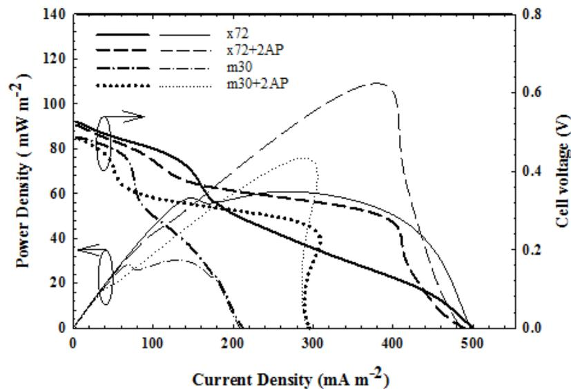
**Fig. 3.** Power density and polarization curves for *Acinetobacter* sp. x72 (x72) and *Enterobacter* sp. m30 (m30) dominant mixed culture MFCs using 2-aminophenol (2AP) at ca. 120 and 170 mg/L as electron shuttle mediator, respectively.
