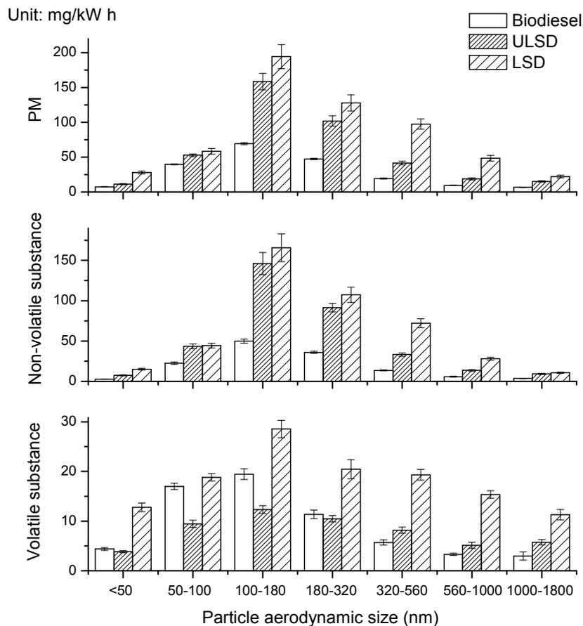
**Fig. 3.** Effect of fuel type on the mass-size distribution of particulate matter (PM), volatile substances and non-volatile substances at 0.7 MPa.
