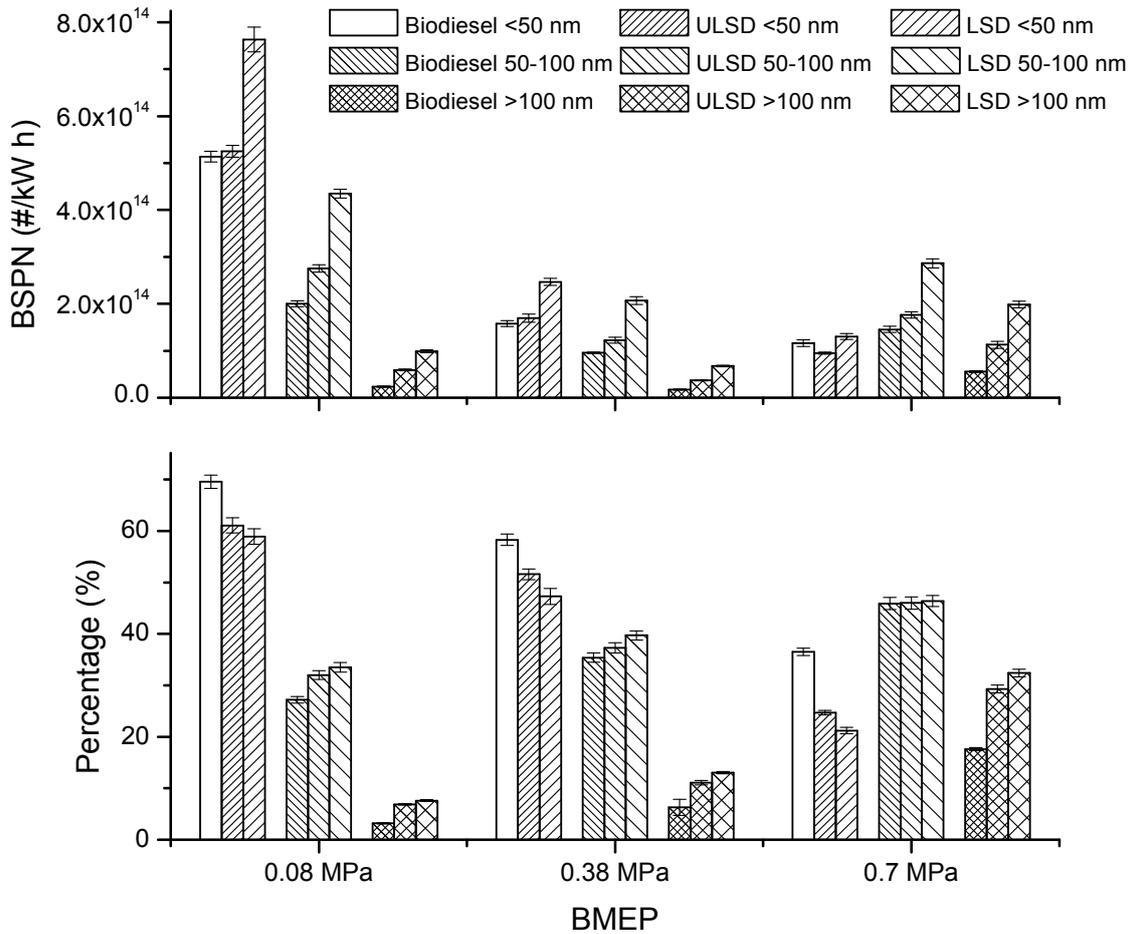
**Fig. 9.** Effect of fuel type and engine load on (a) BSPN (without TD) and (b) number-fraction distribution in different size groups
