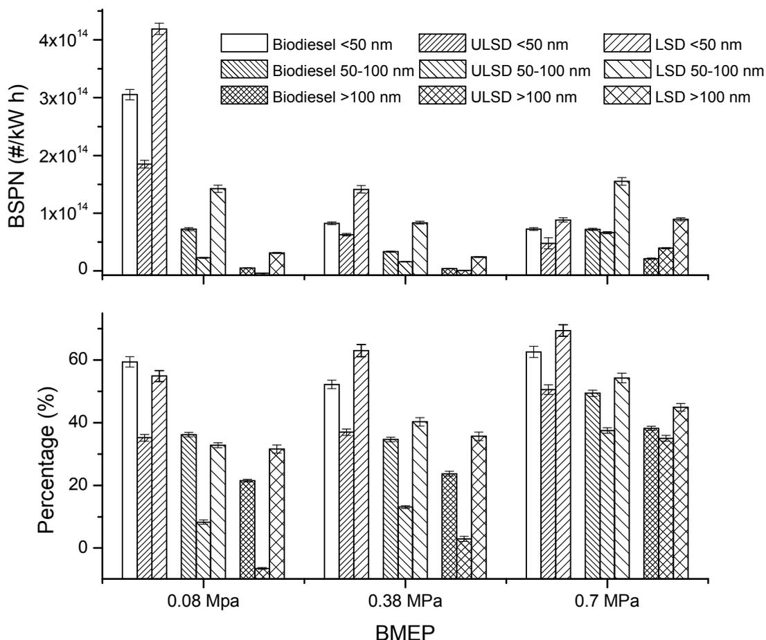
**Fig. 10.** Effect of fuel type and engine load on (a) BSPN of volatile particles and (b) number-fraction distribution of volatile particles in different size groups
