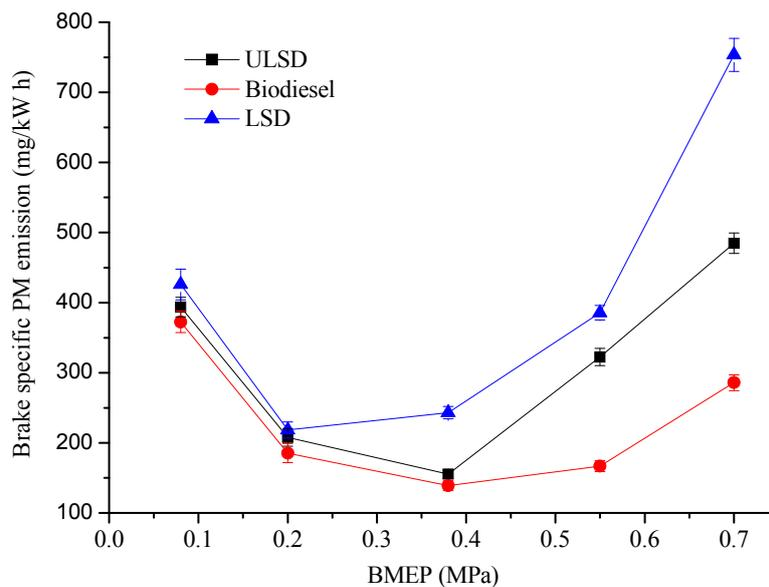
**Fig. 2.** Effect of fuel type and engine load on brake specific particulate emission.
