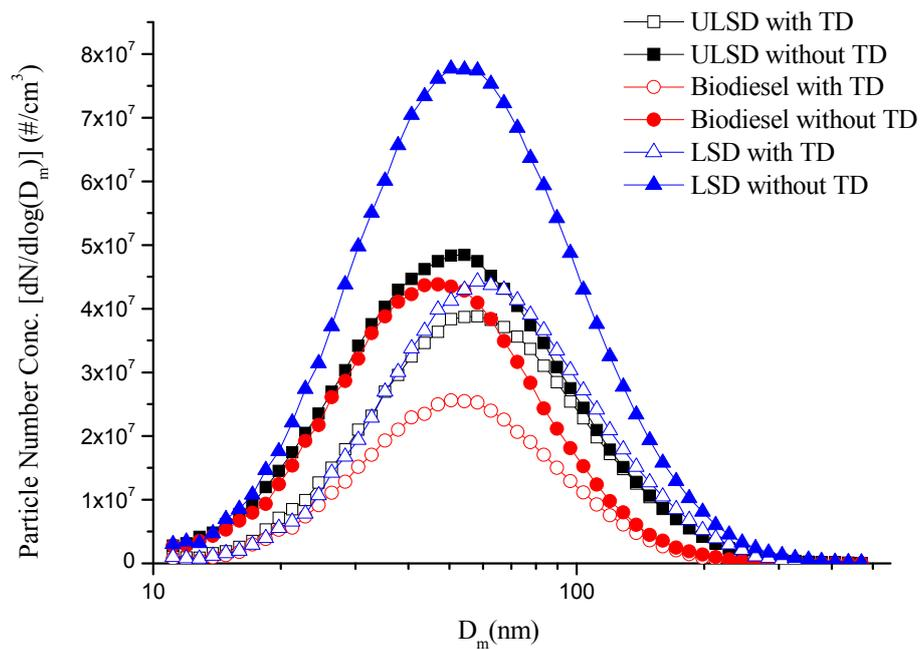
**Fig. 5.** Effect of fuel type and TD on particle number-size distribution at 0.38 MPa.  $D_m$ : mobility particle diameter.
