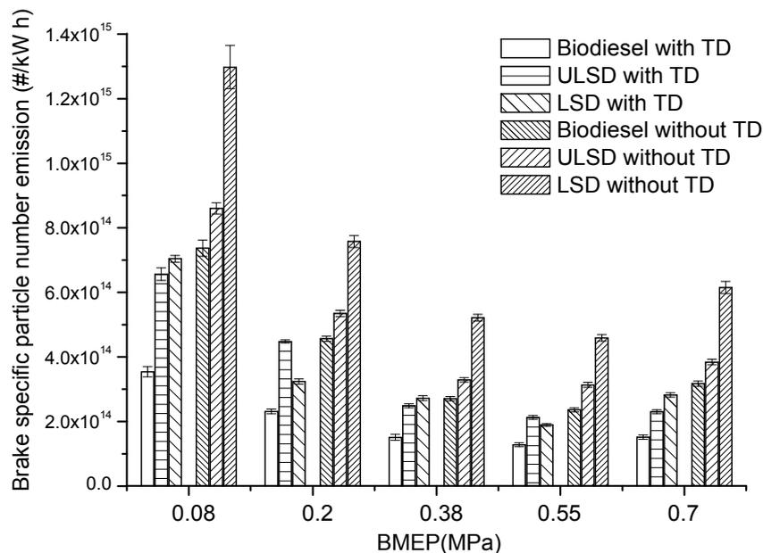
Fig. 7. Brake specific particle number emission with and without TD.
