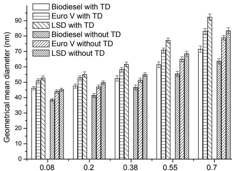
**Fig. 6.** Particle geometrical mean diameter (GMD) with and without TD.
