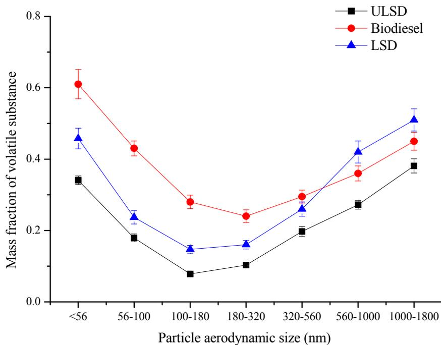
**Fig. 4.** Effect of fuel type on mass-fraction of volatile substances in difference size bins at 0.7 MPa).
