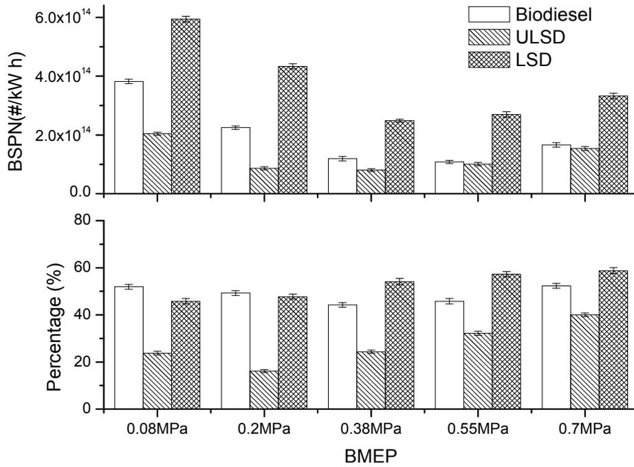
**Fig. 8** Effect of fuel type and engine load on (a) BSPN of volatile particles and (b) number-fraction distribution of volatile particles
