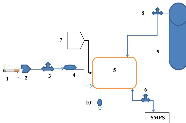
**Fig. 1.** Mainstream cigarette smoke analysis setup 1) cigarette 2) cigarette holder 3) MCS mass flow controller 4) suction pump (1–3 L/min) 5) dilution chamber 6) flow controller for scanning mobility particle sizer (SMPS) 7) Mouth piece for collection of exhaled cigarette smoke 8) N<sub>2</sub> nitrogen cylinder flow controller 9) N<sub>2</sub> cylinder for dilution 10) pump for dilution chamber evacuation.
